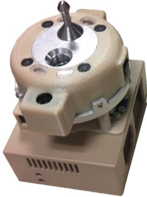
Figure 29: UDP Prototype Mounted to VERTIGO Avionics Stack (Photo Credit: Duncan Miller)
