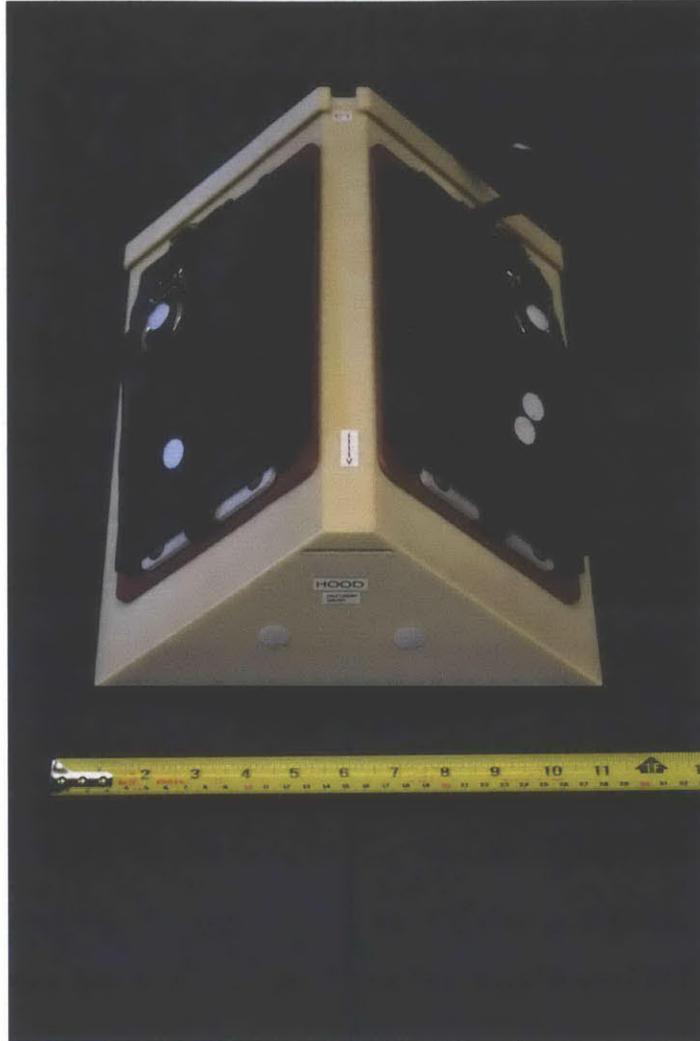
Figure 2-7: Hood with non deployed baffles - front view. Credit: FIT.
