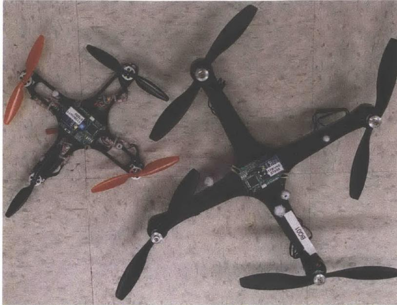
Figure B-1: Two MIT quadrotors equipped to fly in the ACL Real Time Indoor Autonomous Vehicle Test Environment (RAVEN) [54]. The baseline controller on both quadrotors is PID. The small quadrotor uses gains and thrust mappings from the bigger one, resulting in relatively poor trajectory tracking performance.
