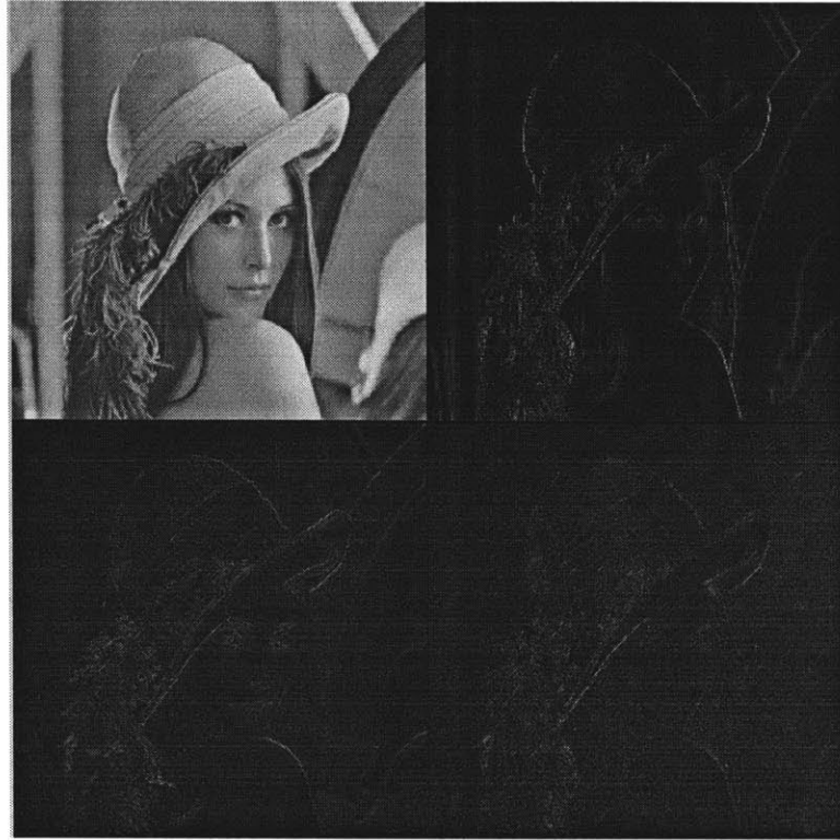
Figure 9. Rate scalability. The upper left corner represents the amount of information contained in the LL layer, and the lower right corner shows the HH layer.
