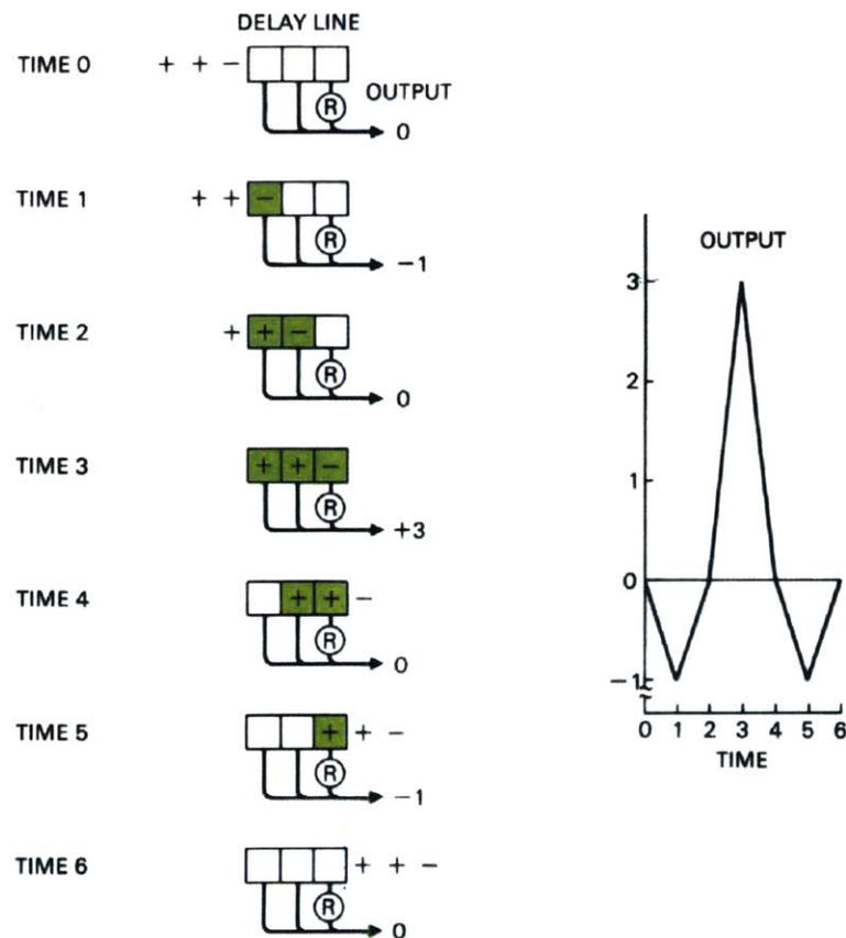
**Figure 2.12** Illustration of Binary Phase Modulation [Stimson, 1998]
