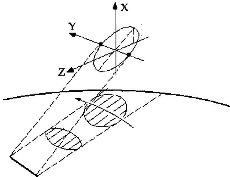
**Figure 3.2** Free Orbit Solution to Hill's Equations
