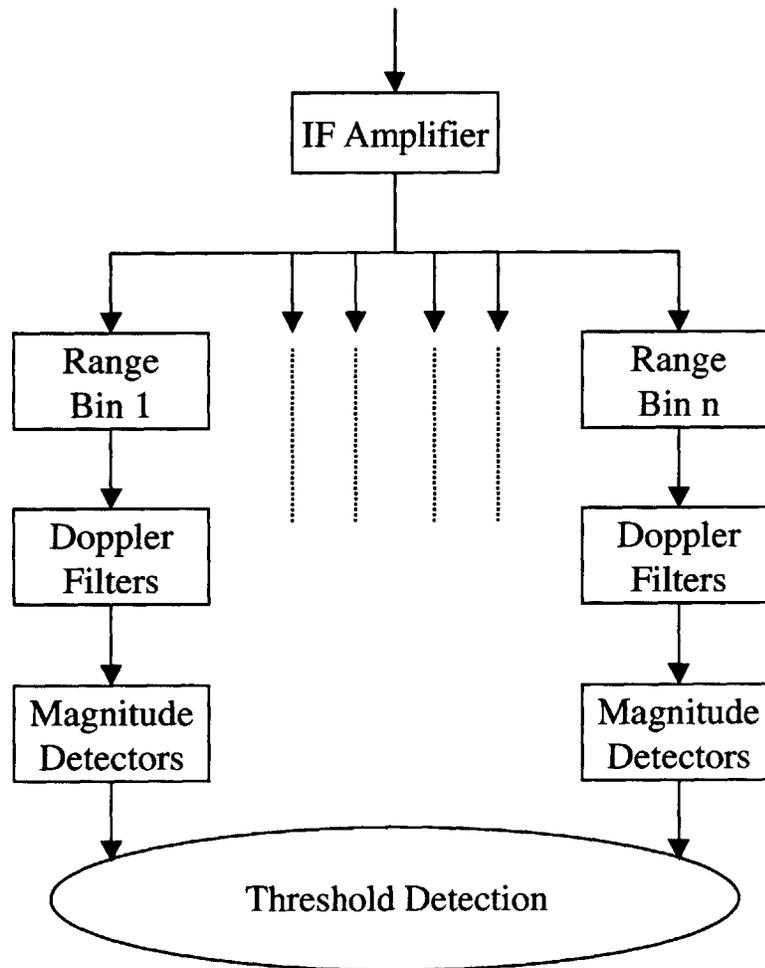
**Figure 2.7** Block Diagram for Radar Signal Processing
