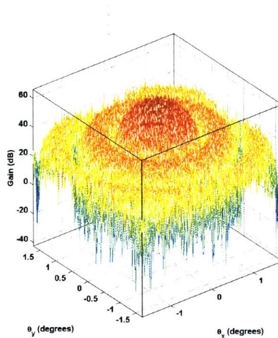
**Figure 4.3** Example Point Spread Function of a Sparse Aperture Interferometer
