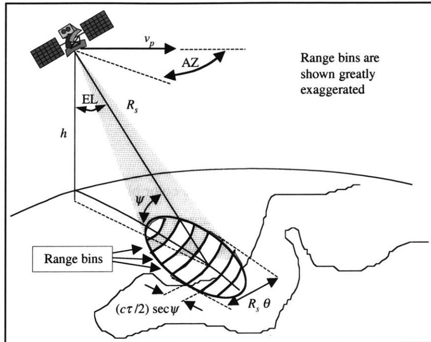
**Figure 2.1** Geometry for a Space-Based Radar System [Shaw, 1998]
