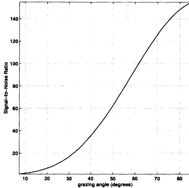
**Figure 4.9** Coverage Area Variations in the Signal-to-Noise Ratio
