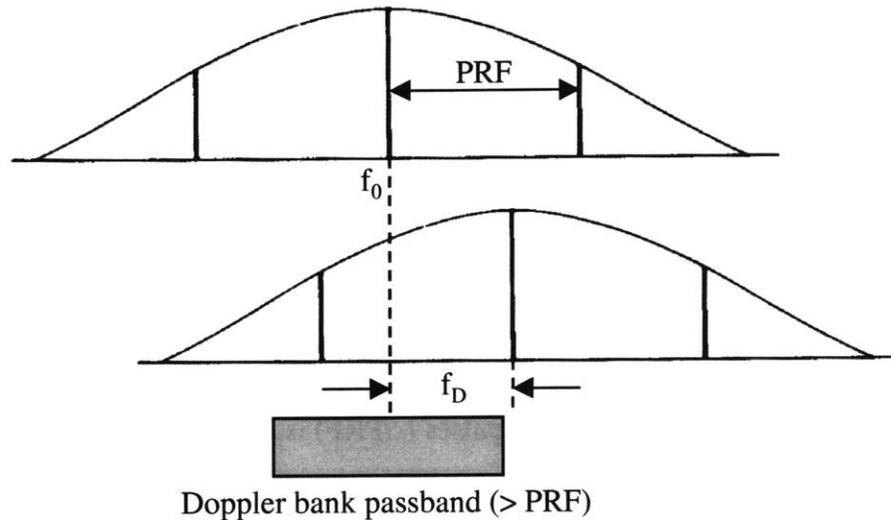
**Figure 2.9** Doppler Ambiguities in the Received Signal Spectrum
