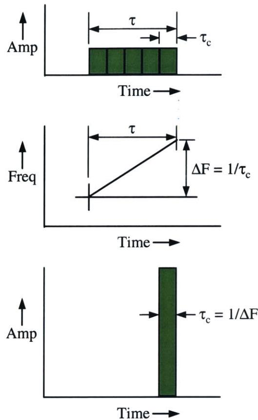
**Figure 2.11** Compressed Pulse in Linear Frequency Modulation
