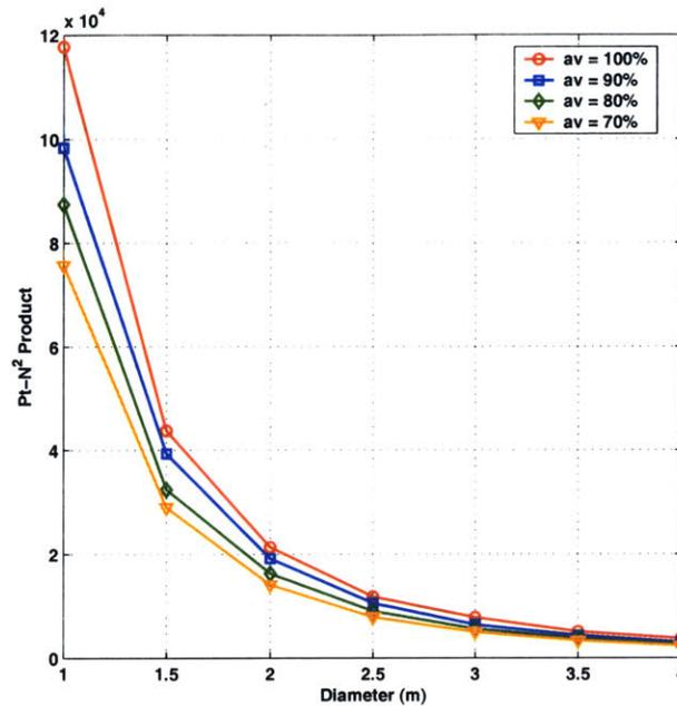
**Figure 5.4** Acceptable System Design Architectures ( $P_d = 85\%$ )
