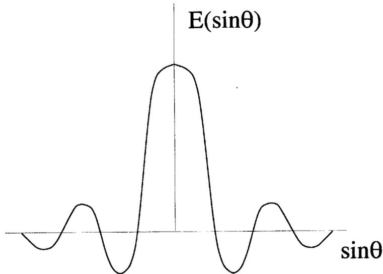
**Figure 2.4** Lobe Structure of the Antenna Beam
