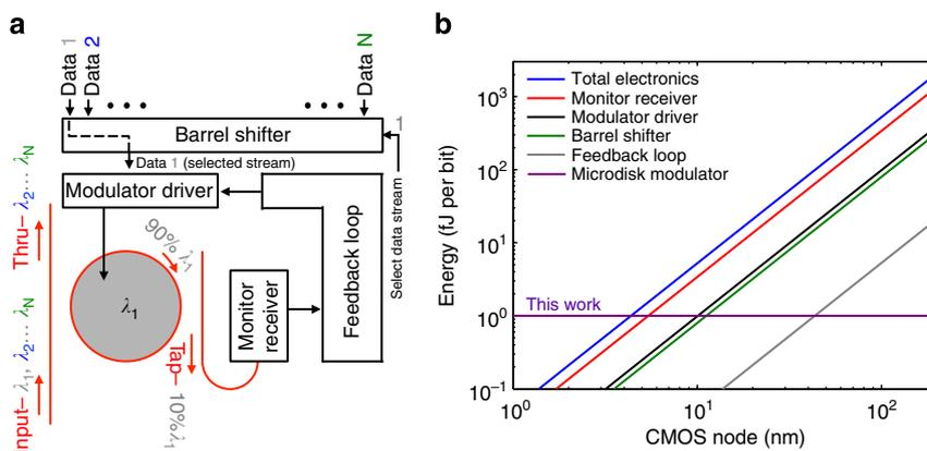
**Figure 6 | Integrated modulator components and energy scaling.** (a) A diagram of the required integrated electrical circuitry to drive, and control the modulator and barrel shifter to correct for channel hopping between modulators. (b) The energy consumption scaling of the modulator subsystem is plotted as a function of CMOS node scaling, showing sub-fJ per bit driver and total electronics energy at advanced CMOS nodes.
