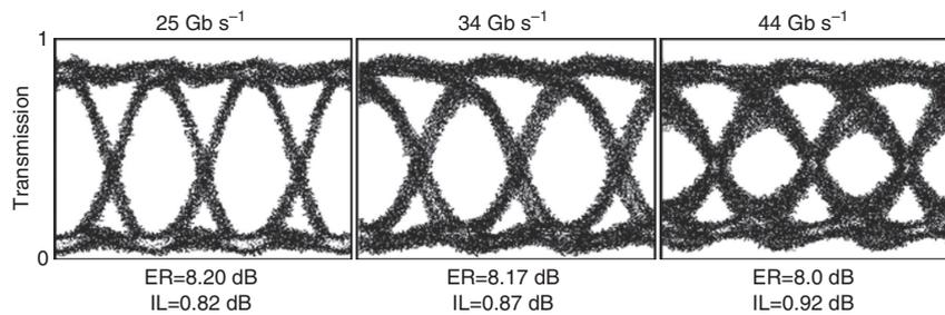
**Figure 7 | Bandwidth-limited data transmission.** The experimentally measured high-speed optical eye diagrams of the silicon microdisk modulator when driven by a terminated probe and a 2.2 V<sub>pp</sub> NRZ-OOK PRBS with a pattern length of 2<sup>31</sup>-1 at data rates of 25-, 34- and 44 Gb s<sup>-1</sup>. The extinction ratio (ER) and insertion loss (IL) are denoted below the eye diagrams at each data rate.
