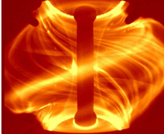
Figure 1-3: An ELM crash on the Mega Amp Spherical Tokamak in Culham, UK. Used with permission from, and photo credit to, Culham Centre for Fusion Energy, http://www.ccfе.ac.uk/ , [14].
