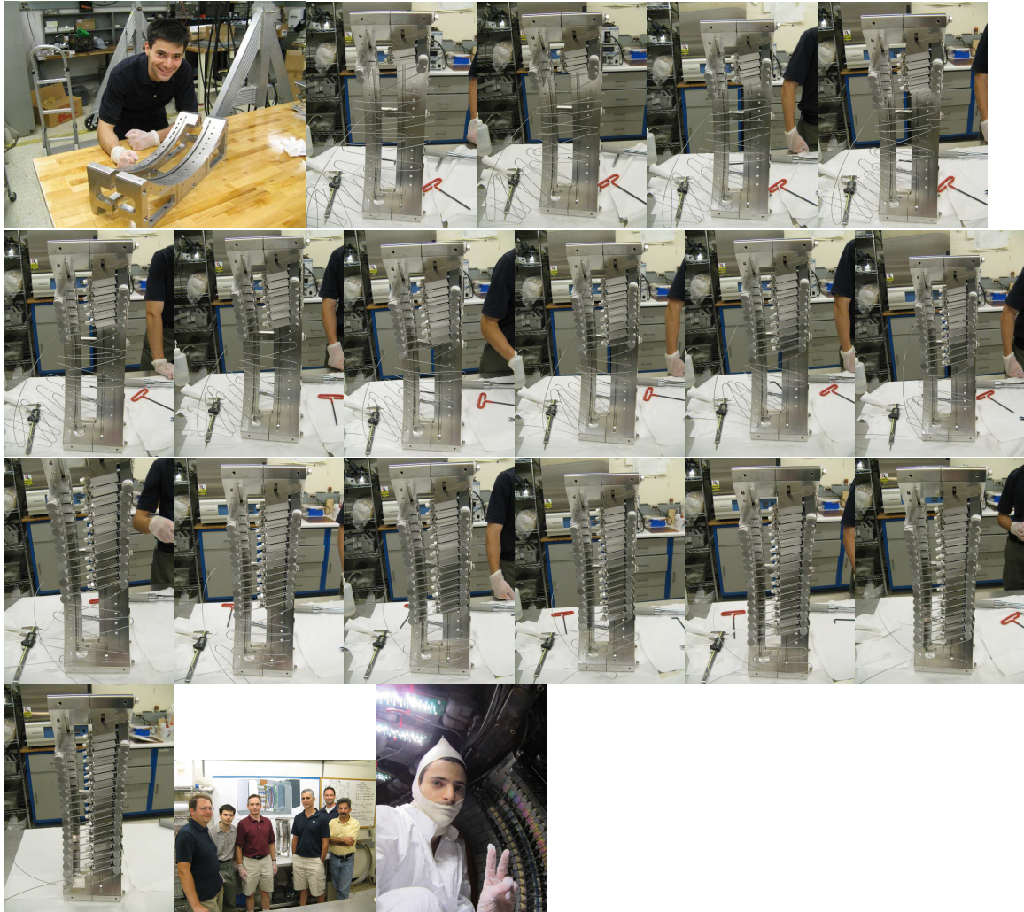
Figure G-1: Sequence of winding the Shoelace antenna. The wire was first bent into shape on a separate, flat, full-size winding fixture mock-up, then unwound from this fixture and transferred to the real antenna. (Photo Credits: B. LaBombard, T. Golfopoulos)
