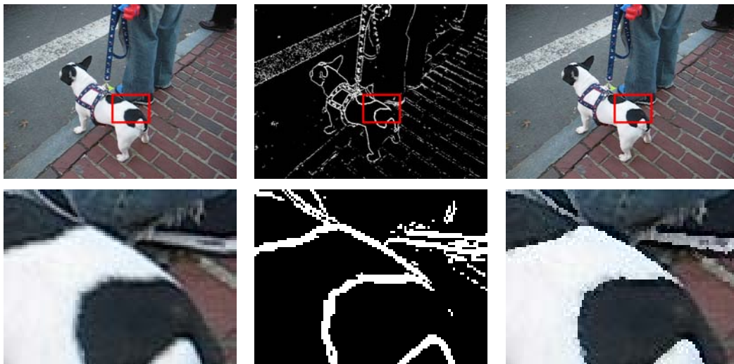
Figure 4.7: Visualization of the edge sharpening. Original image (left), edge detection (middle), edge sharpened image (right). Bottom row shows a detail of the image.
