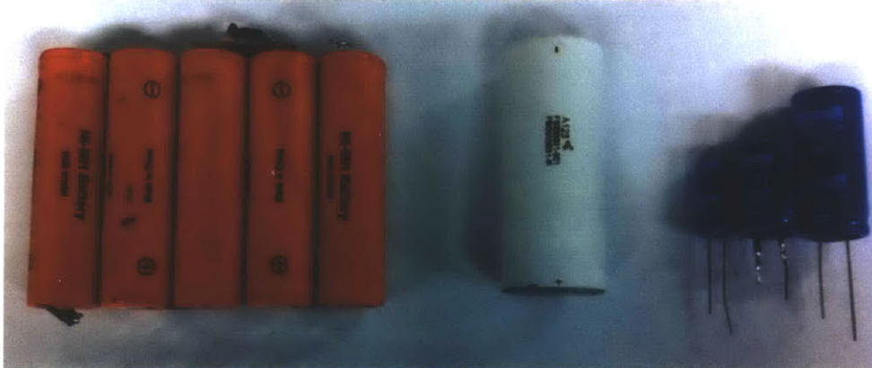
Fig. 3- 6 Devices used in the investigation Ni-MH battery pack, Lithium-ion battery pack and ultracapacitor cell (left to right: 5F, 25F, 50F)
