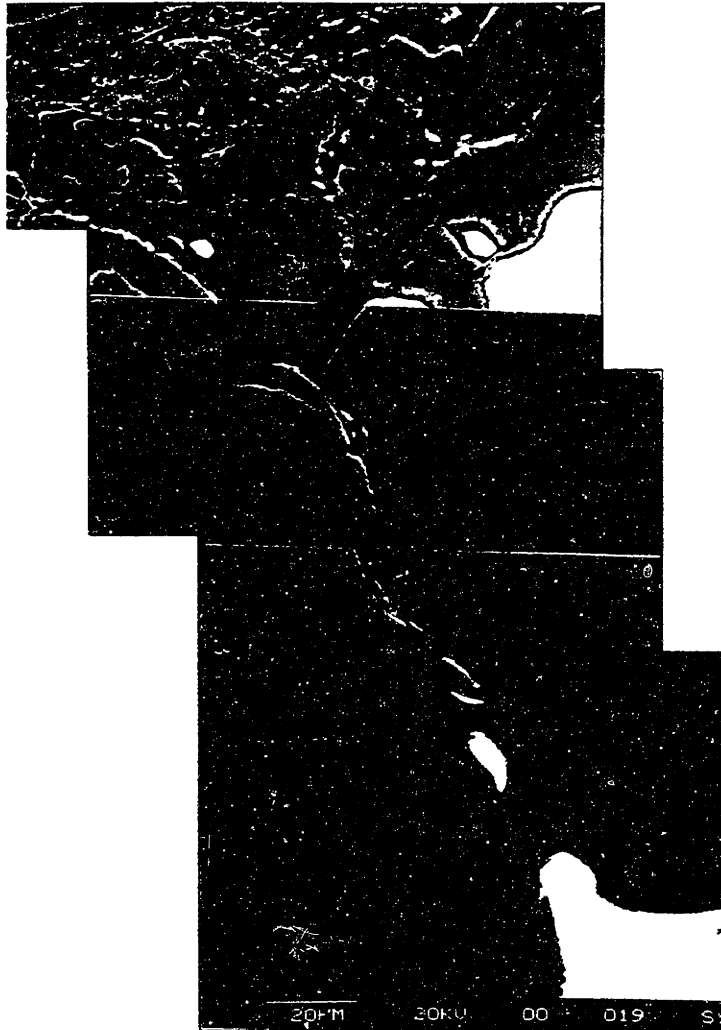
Figure 2-1 A through-wall crack in a 1/16-in Hastelloy C-276 preheater tube exposed to a feed of \text{CH}_2\text{Cl}_2 for 40 h. The top of the photo is the inner surface of the tube, while the outer surface is at the bottom. From Mitton et al. (1995).
