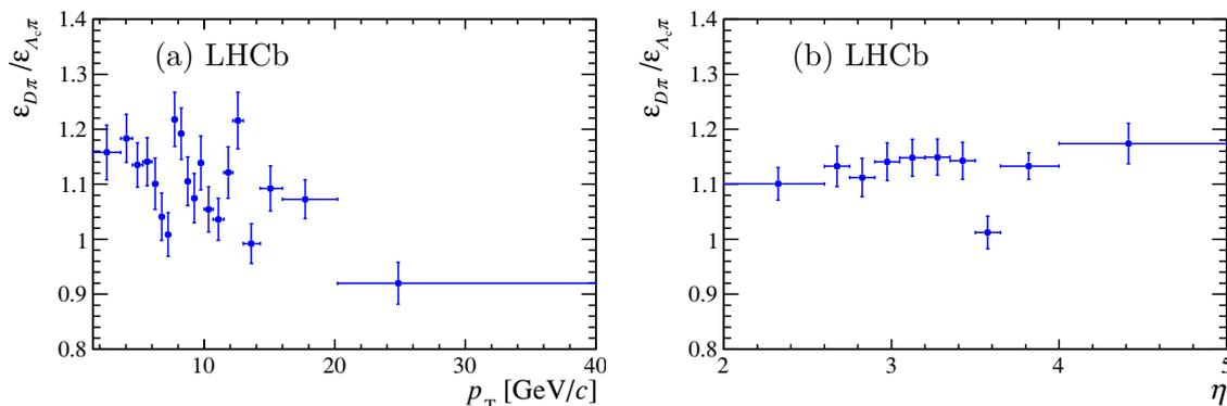
**Figure 1.** Ratio of total selection efficiencies in bins of the (a)  $p_T$  and (b)  $\eta$  of the  $b$  hadron. The horizontal error bars indicate the range of each bin in  $p_T$  or  $\eta$  respectively.
