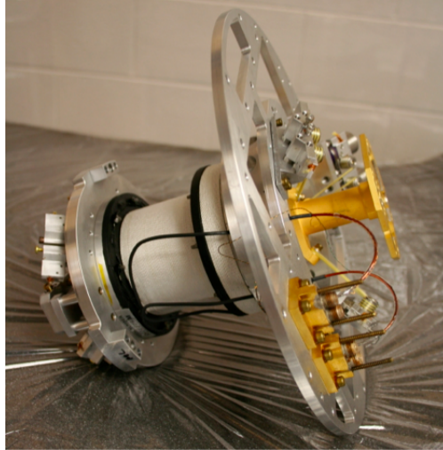
Figure 4-7: A picture of the insert with the suspended mass installed with kevlar strings. The magnet leads run to the high current connectors toward the bottom of the image. The aft side of the insert is on the right side of the image while the forward side, which sits inside the helium can bore is on the left side of the image. The detector box, 2 K thermal shield, magnetic shield, and 2 K electronics are not installed in this image.
