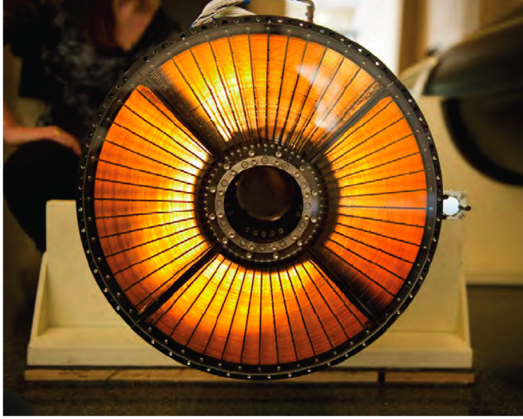
Figure 4-39: A picture of the Micro-X mirror from the aft side (where X-rays enter). The mirror is illuminated from the back with a flashlight, revealing the color of the gold-coated foils.
