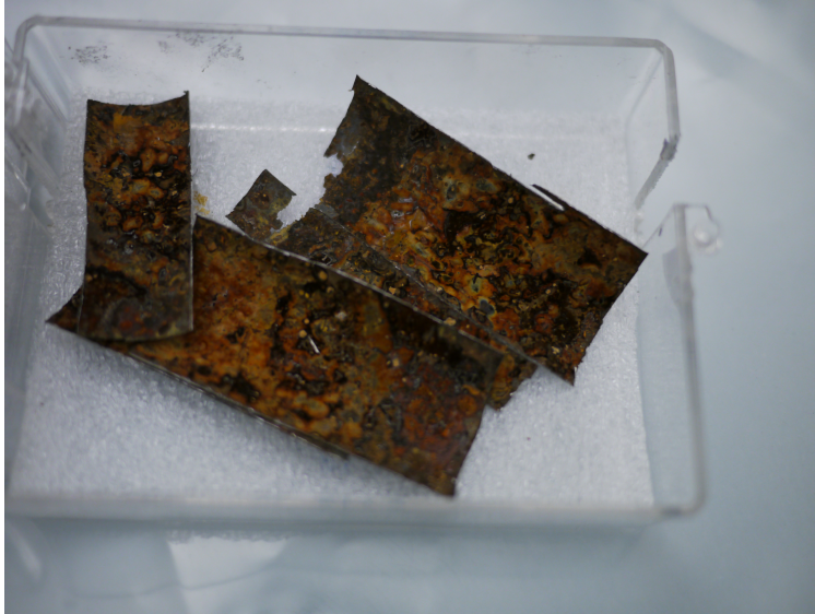
Figure 4-10: The inside of the stainless steel enclosure of the third salt pill after it was cut off of the gold wire cage. We suspect contamination during machining combined with the use of 304 stainless steel rather than 316 stainless steel caused the salt to corrode the tube to the point of mechanical failure.
