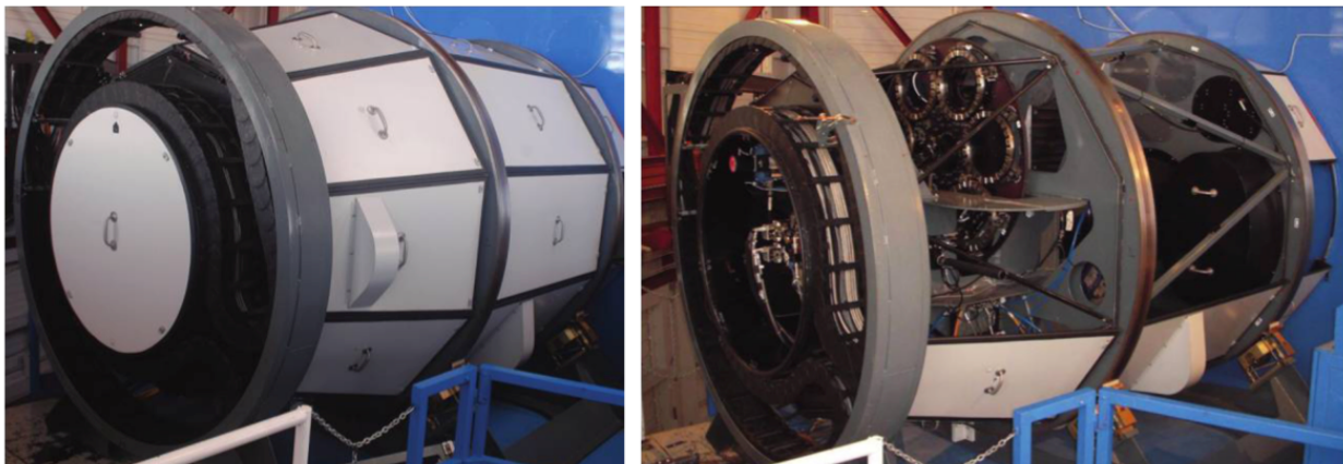
Figure 2-5: Pictures of the IMACS instrument with (left) and without (right) the instrument covers, mounted on the Baade telescope (reprinted from [28].)
