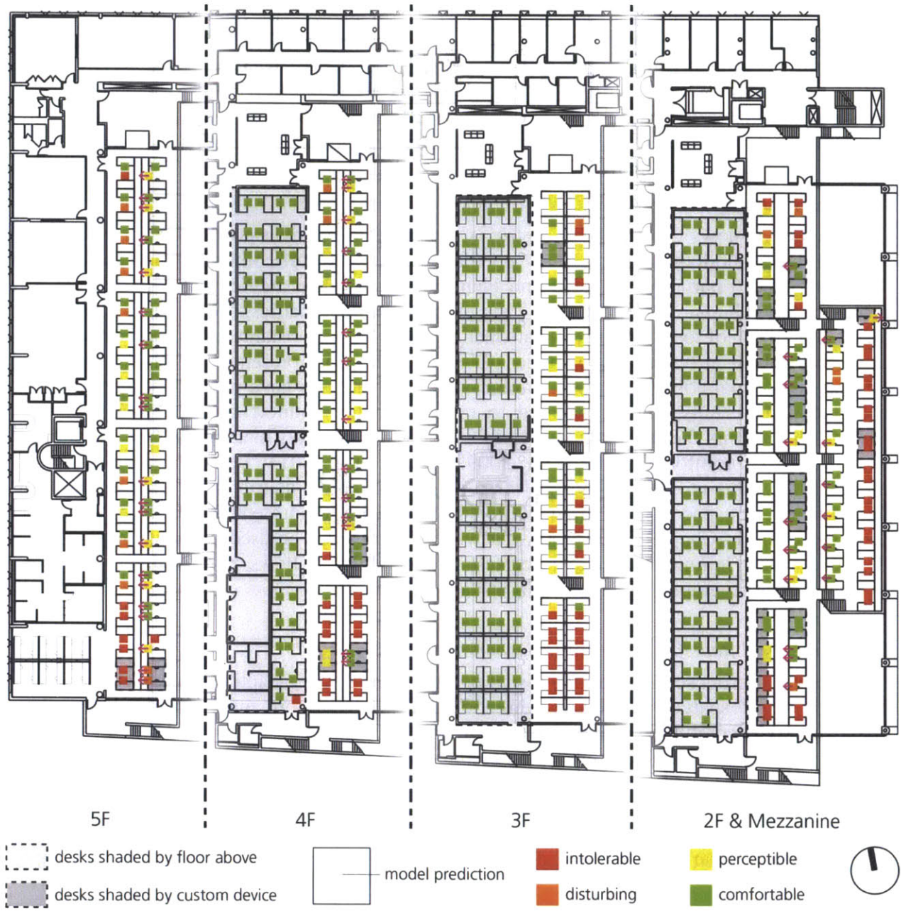
(b) Seating position based on side table orientation potential to increase predicted comfort. Figure 8.5 Comparison of morning predicted satisfaction for two seating layouts in Gund Hall.
