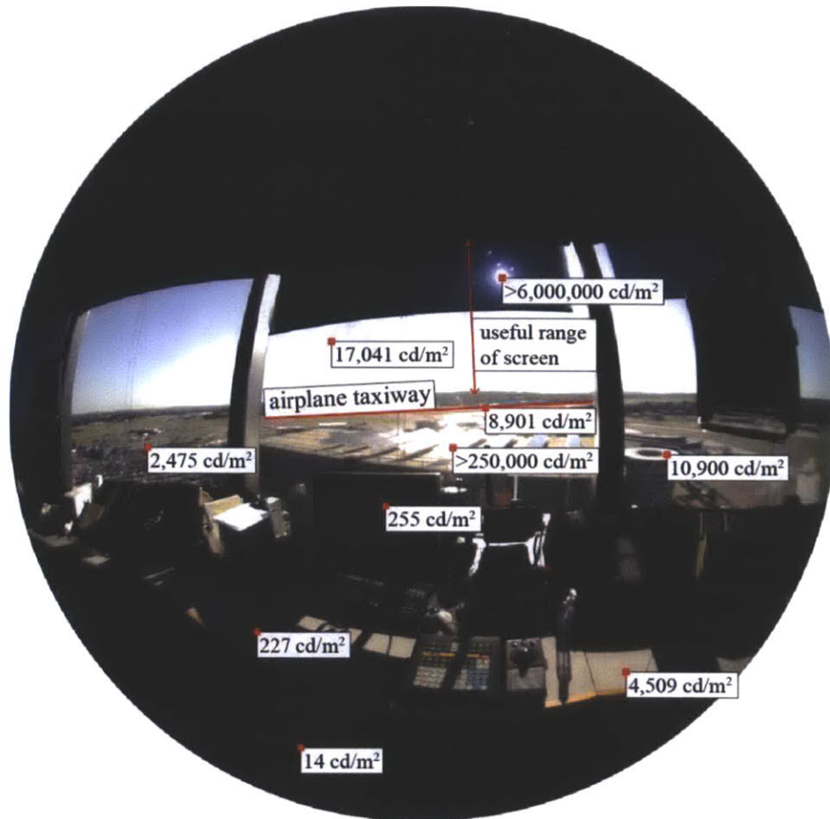
Figure 7.1 High dynamic range photograph of glare problem taken on August 30 th , 2013 at 7:22 solar time.
