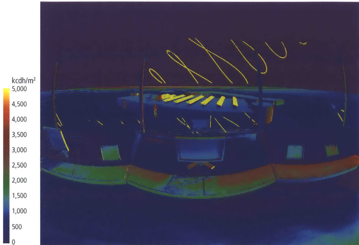
Figure 8.4 Annual contribution of direct sunlight illustrating that further investigation into reflections from the PV array are warranted.
