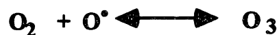
Figure 4.1: The equilibrium reaction between ozone and oxygen/atomic oxygen and oxygen containing free radicals.
