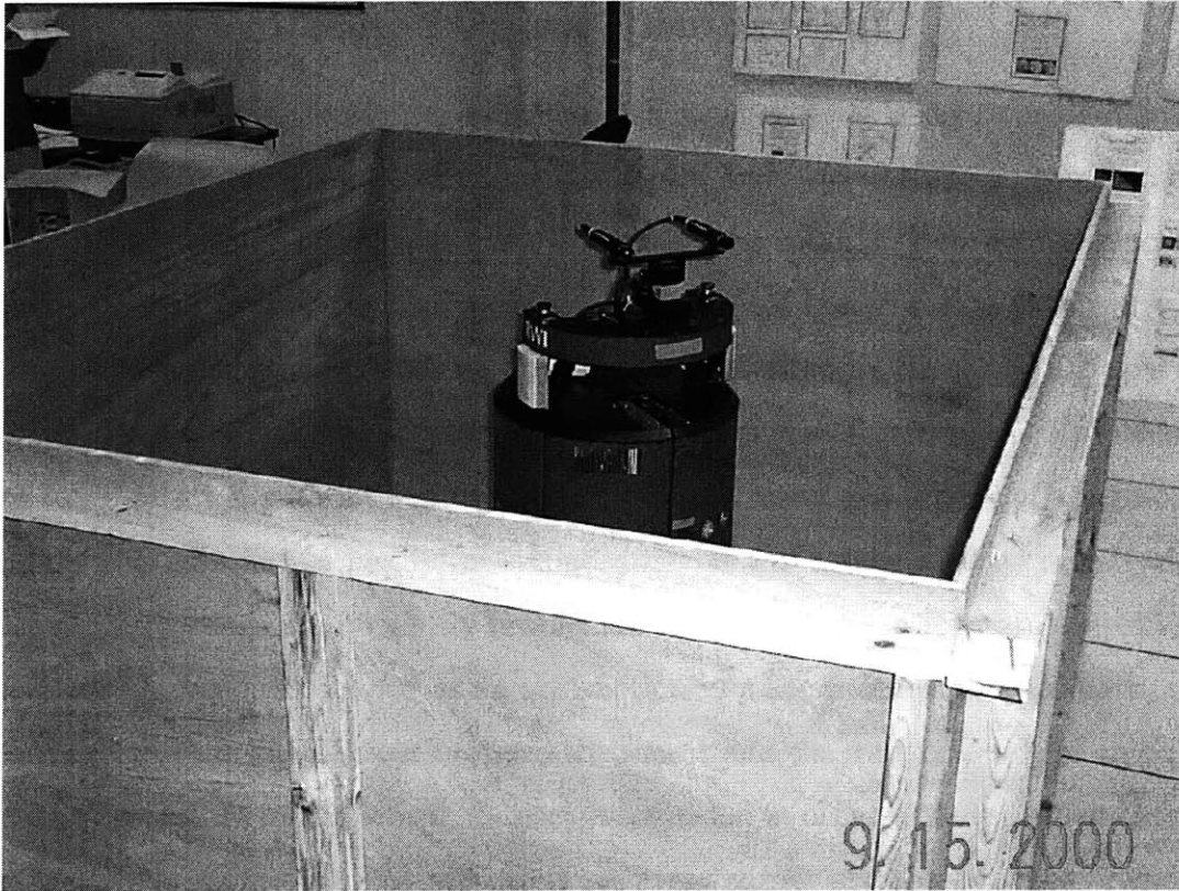
Figure 1-1: The B21 mobile robot (illustrated here in the plywood box used for simple testing of the algorithm.)
