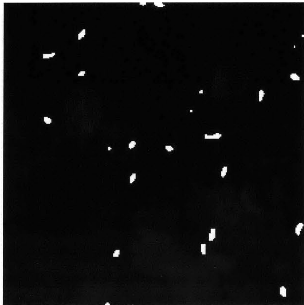
Figure 5-14: The image of Figure 5-13 after dilation of each point to a square of dimensions 0.16 mm x 0.16 mm
