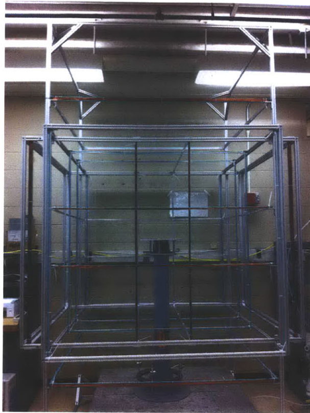
Figure 3-8: MIT Space Systems Laboratory's Helmholtz Cage [37]
