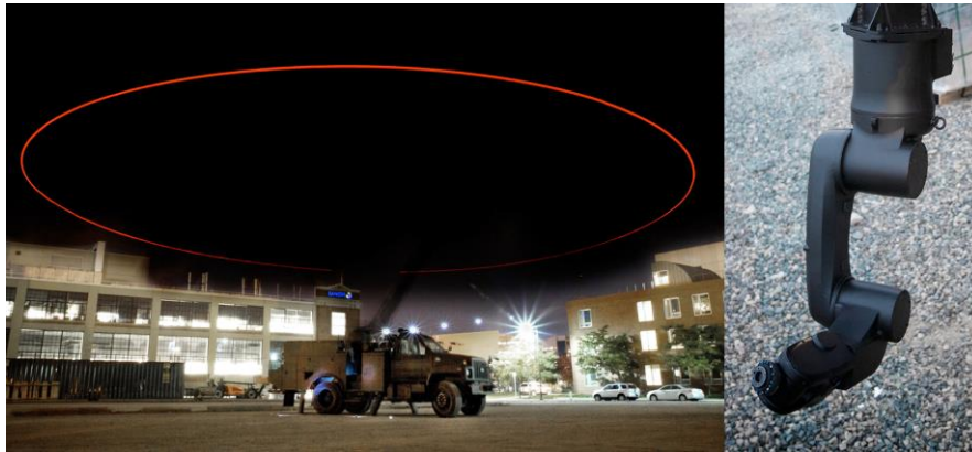
Fig. 2. The range of motion for the DCP is shown through long-exposure photography (left). The DCP uses a combination system of a 5-axis Altec hydraulic boom arm and a small 6-axis KUKA robotic arm (right).
