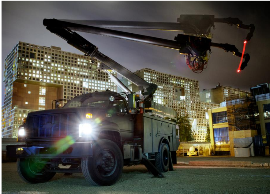
Fig. 1. The Digital Construction Platform (DCP) is comprised of a 6-axis KUKA robotic arm mounted to a 5-axis Altec hydraulic boom arm.
