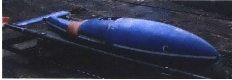
Figure 1-13: The first generation robotic dolphin with pneumatics. – Motomu Nakashima
