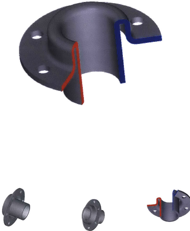
Figure 3-11: Drawings of the pitch seal boot. The large lift and thrust forces cantilevered out on the foil result in radial deflections of the shaft attached to the foil. In order to prevent these radial deflections of the shaft from transmitting large loads to the shaft seal, this seal boot allows the shaft seal to ride on the shaft and the deflections are taken up in the compliance of the boot. These deflections are on the order of several millimeters. While these deflections may seem small, o-ring seals need tolerances on the order of 0.01 millimeters. These seal boots are made of a flexible urethane with a Shore A hardness of 70. The depth rating for this seal has not been measured, but it will be on the order of 10 meters. Fatigue is not an issue with these seals because the small motions of the boot.
