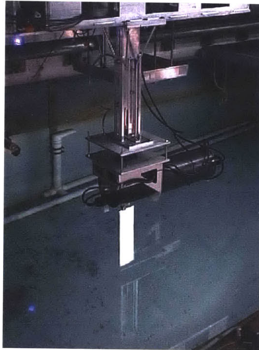
Figure 4-1: Two housing foil actuator mounted to the six axis dynamometer.
