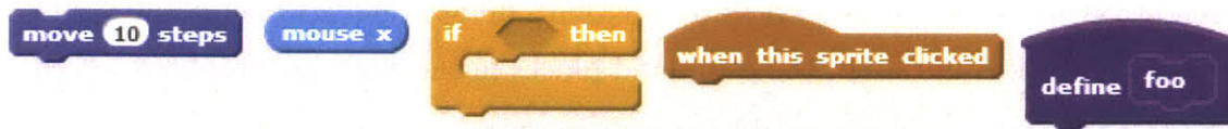
Figure 2-2: From left-to-right are samples of command , function , control structure , trigger , and definition blocks.
