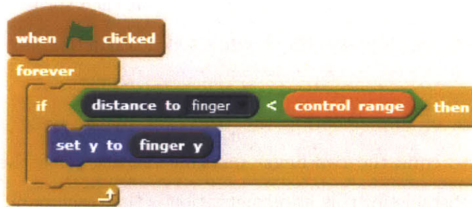
Figure 4-4: Here is a sample script for controlling the paddle in a basic two-player Pong game using the Closest Finger Design.
