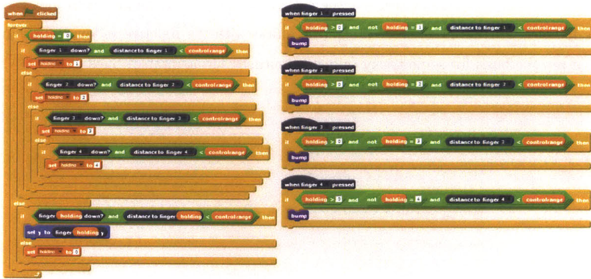
Figure 5-7: Here is a sample script for controlling the paddle in an advanced two-player Pong game using the Relative Indexing Design.
