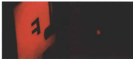
Figure 6-4 Test of the telescope demagnification The image of the, 'f', is demagnified ten times (and inverted) through the telescope.
