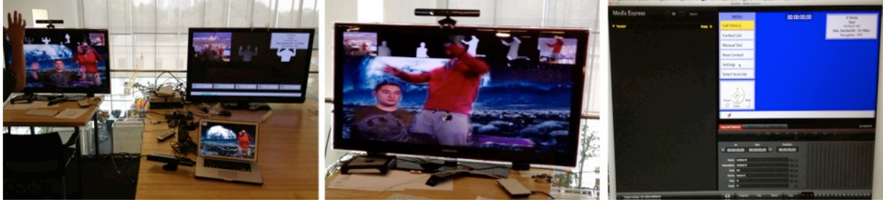
Figure 65. HDVC setup testing in the lab. The depth image is baked into the 1080p stream and routed back to the PC.
