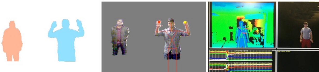
Figure 38. A user masking contour, skeleton and hand tracking, and gesture recognition based on skeleton data.
