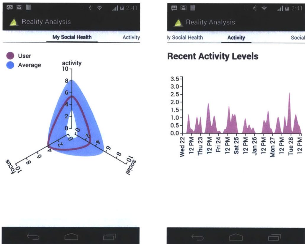
Figure 4-5: Social Health Tracker provides a view of 3 metrics: activity, focus, and social on a personal (pink) and average (blue) level. These metrics are calculated from sensor data, aggregated in a privacy-preserving fashion, and presented as a current score as well as historical levels over time.
