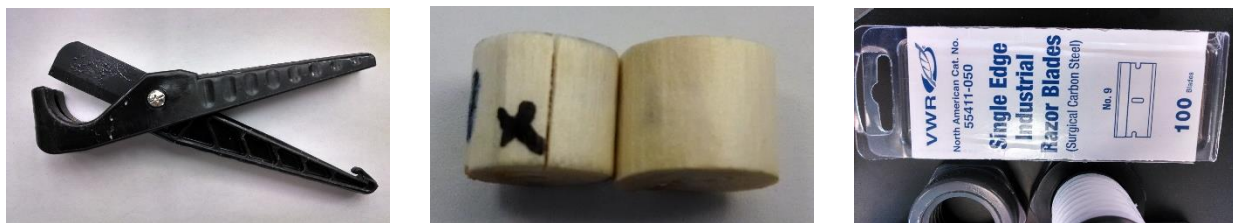
Figure 3-4 (Middle) Two samples cut with (Left) Kwik Cut pipe cutter and (Right) industrial razors, the left sample has a crack through the center of it, compromising it's capability as a filter
