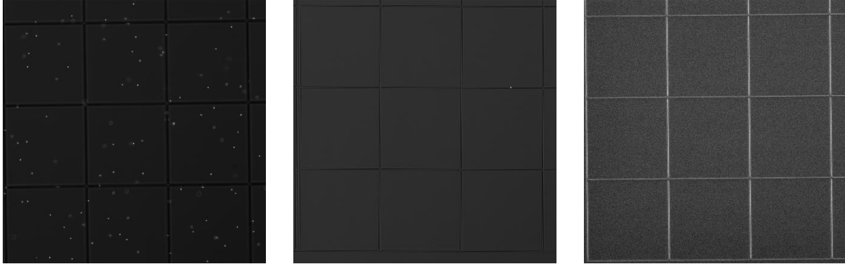
Figure 5-10 Fluorescent microsphere concentrations in (Left) unfiltered feed solution (Middle) filtrate from 0.10in sample (Right) filtrate from 0.25in sample. This suggest that the minimum length to rejection 1 \mu\text{m} is 0.25in. (Not Shown) filtrates from the 0.41in, 0.51in, 0.77in, and 1.00in because they were identical to the 0.25in filtrate. Each box is 0.25mm x 0.25mm.
