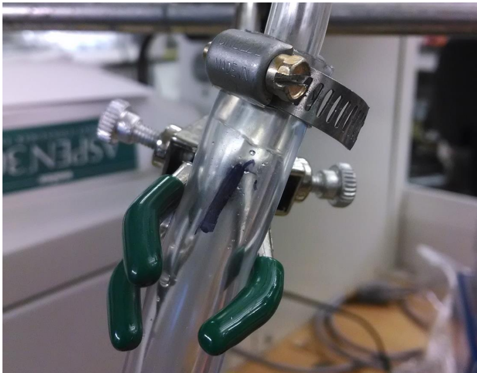
Figure 8-3 Modified experimental setup with hose clamp at connection between Nitrogen tank and xylem filter.
