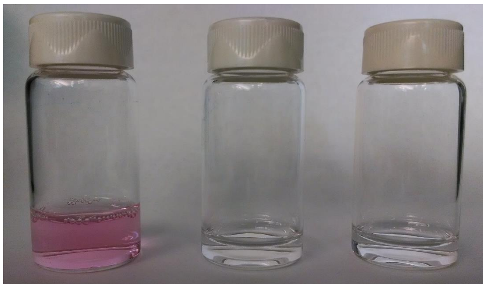
Figure 8-7 (Left) Unfiltered red ink at 5,000x dilution (Middle) Ink filtered using sample that was rewet after being coated with MW 10K PVP and (Right) MW 40K PVP
