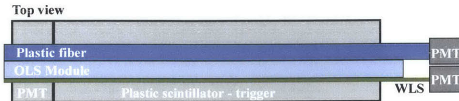
Figure 5.1. OLS module versus plastic fiber muon detection efficiency experimental setup. All plastic scintillator (1" x 1" x 4") events above 200 mV triggered the collection of the OLS module and plastic fiber signal. All OLS module and plastic fiber events above 30 mV were counted as muon events.
