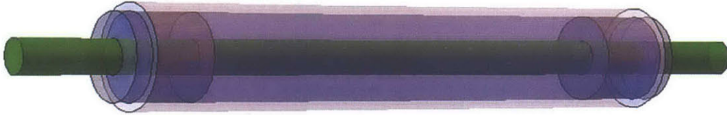
Figure 3.16. Example of modeled configuration with 2mm diameter WLS inside OLS filled AWG4 PTFE tube.
