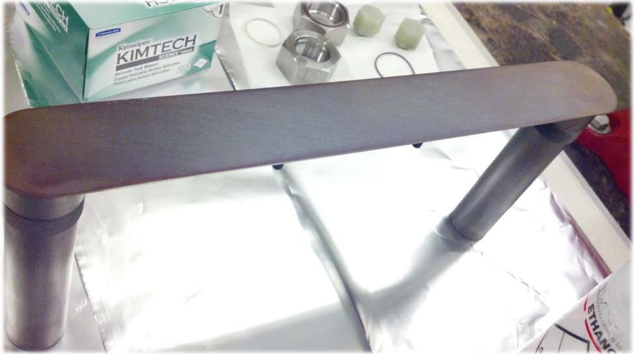
Figure 104: Heater Plate Following Surface Finishing Followed by Oxidation in Air at 600 °C.
