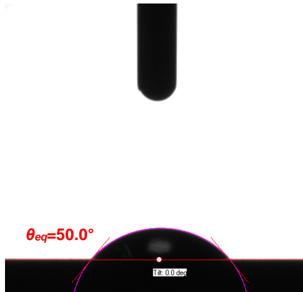
Figure 160: Equilibrium Contact Angle of De-ionized Water on Well-wetting (Oxidized) 316 Stainless Steel Heater Surface.
