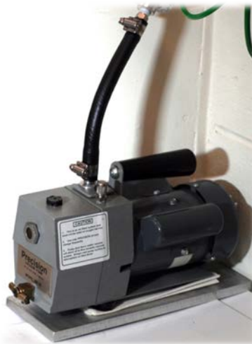
Figure 44: Vacuum Pump Installed in the Flow Facility.
