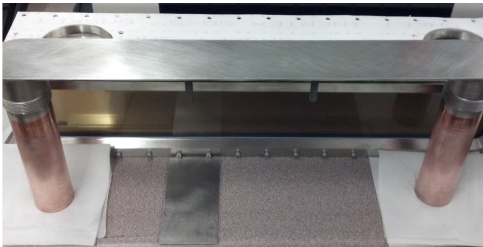
Figure 78: Photograph of Heater Plate Following Surface Finishing with Sample Coupon on Table.
