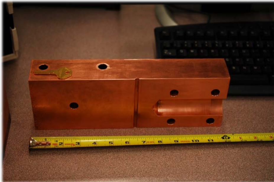
Figure 18: Electrode Clamp Used to Connect the Conductors to the Test Section.
