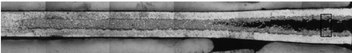
Figure 7: Micrograph of Failed IRIS-2 Plate. The plate consisted of atomized U-7Mo dispersion fuel in an aluminum matrix, clad in aluminum, loaded to 8.3 gU/cm 3 . Peak cladding temperature and heat flux were 93 °C and 2380 kW/m 2 , respectively. Failure was likely initiated by interdiffusion of U-Mo and Al. Source: Ref. [11].
