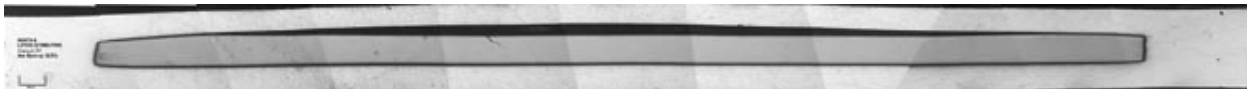
Figure 8: Micrograph of a U-10Mo Monolithic Fuel Plate from the RERTR-6 Test. The clad delaminated from the fuel following irradiation due to poor bond strength between the clad and fuel, likely due to interdiffusion. Source: Ref. [11].
