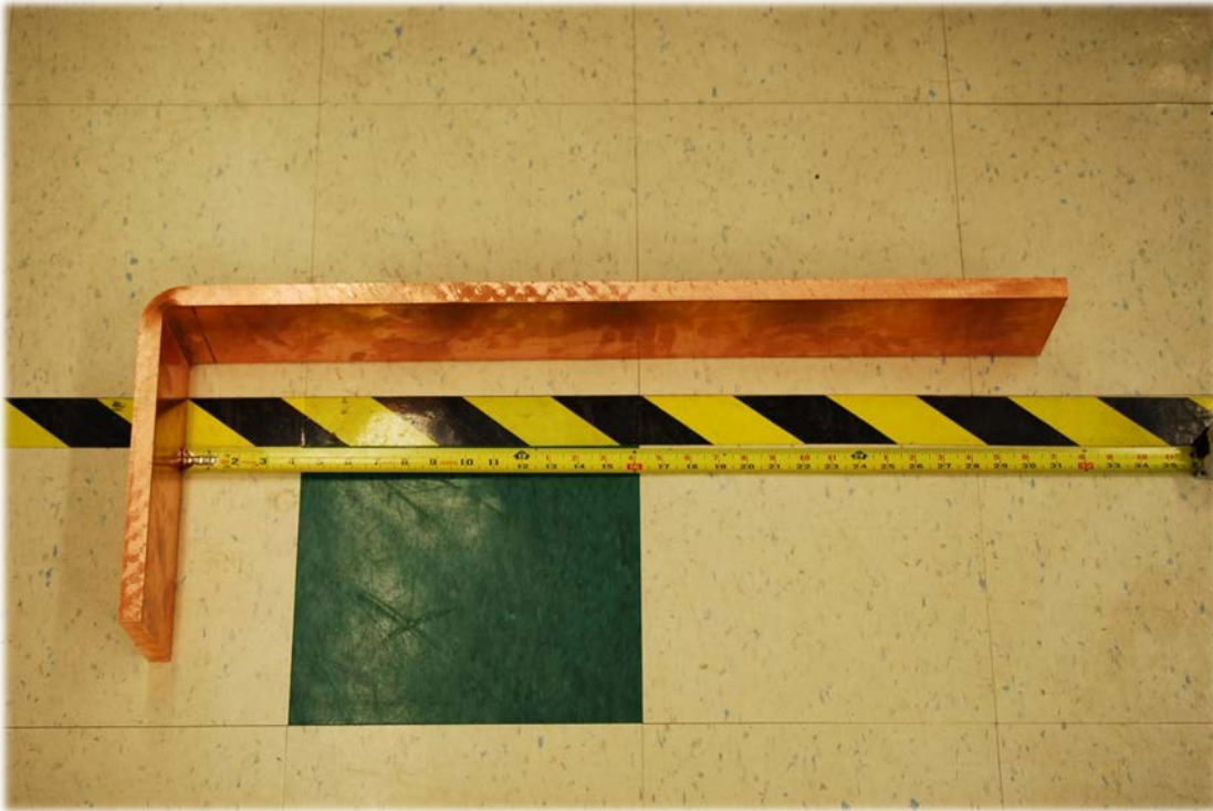
Figure 19: Copper Busbar for Connecting the Positive Electrode of the Power Supply. The bar was bent using a hydraulic roll bender.
