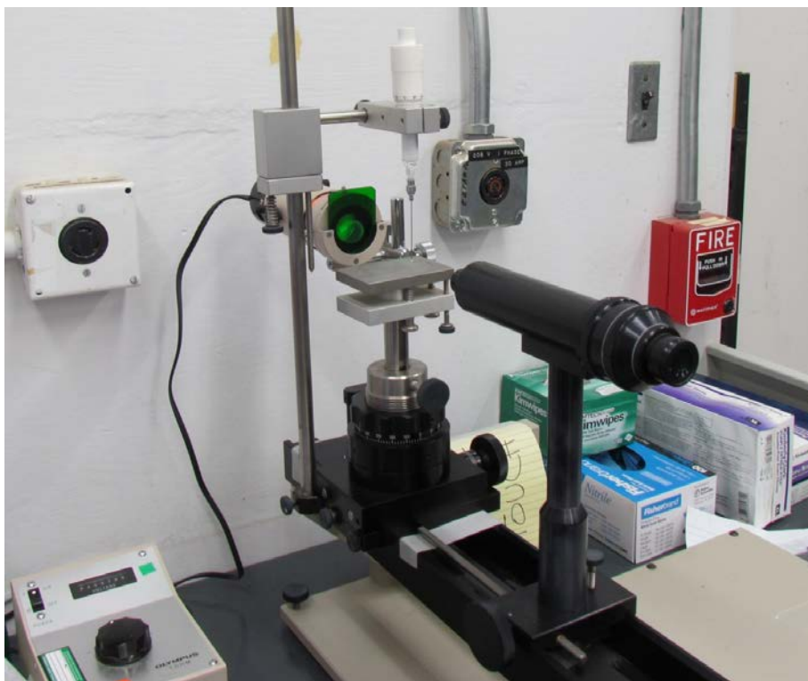
Figure E15: Goniometer for Performing Contact Angle Measurements. Although no optical software was available, accurate results were achievable with the “manual” setup for sessile drop measurements.
