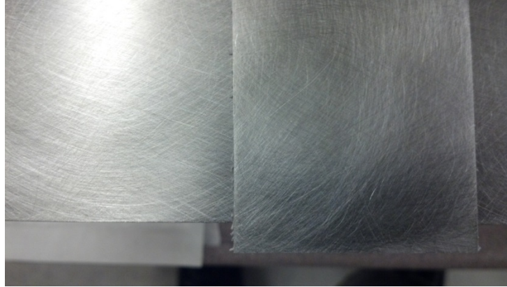
Figure 79: Close-up Comparing Heater Plate Surface (left) to Sample Coupon Surface (right).
