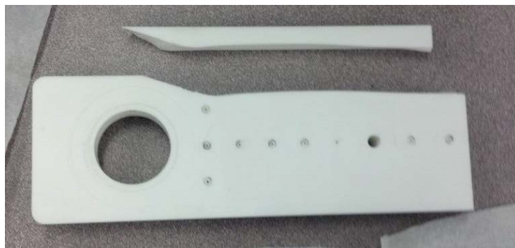
Figure 20: Section of Failed Macor Insulator.
