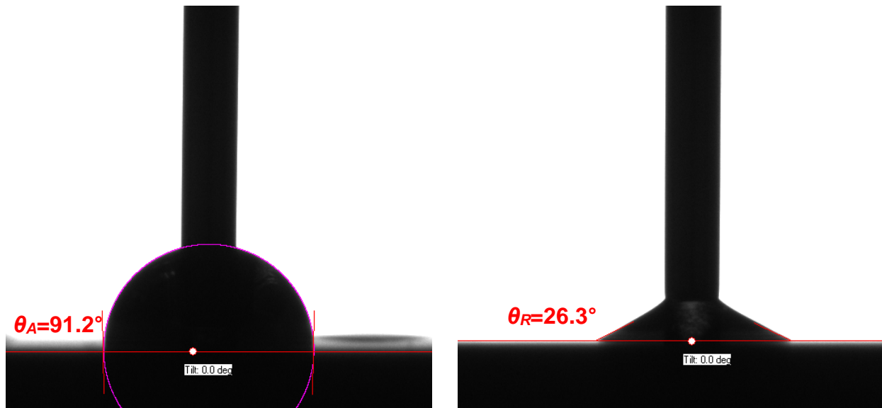
Figure 159: Static Advancing Contact Angle (left) and Static Receding Contact Angle (right) on Nominal 316 Stainless Steel Heater Surface.
