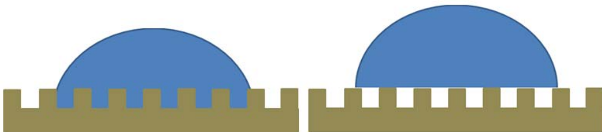
Figure 141: Wetting in the Wenzel State (left) and in the Cassie-Baxter State (right). In the Wenzel regime, a liquid droplet impregnates surface features, typically resulting in contact line pinning, contact angle hysteresis, and roll-off resistance. In the Cassie-Baxter regime, air pockets remain below the liquid droplet, resulting in a higher roll-off tendency.
