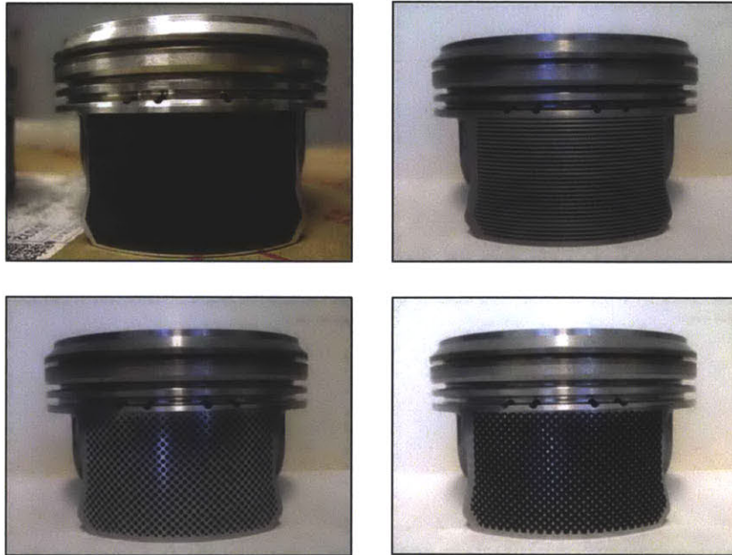
Figure 4.1 – Piston's skirt pattern prototyped
