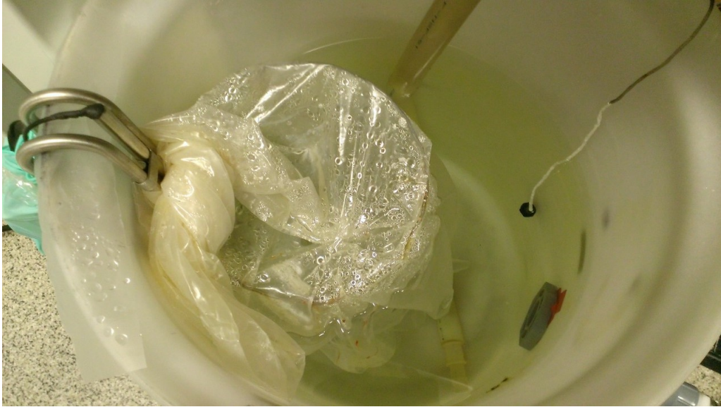
Figure 3-19: Heater separated from feed tank using a plastic bag
