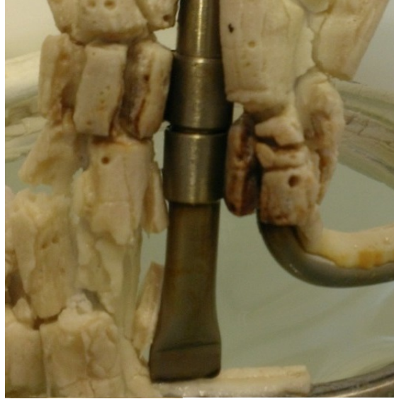
Figure 3-17: Rust seen on heater element in \text{CaSO}_4 supersaturation experiments
