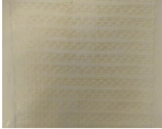
Figure 3-18: Membrane used for experiment (Fig. 3-10) showing discoloration
