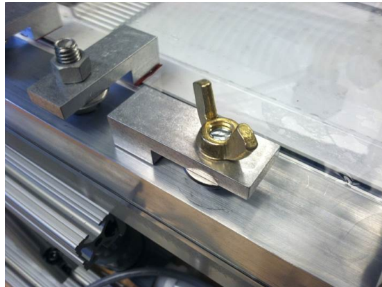
Figure 3-5: Design of quick release clamps for easy access to membrane between tests
