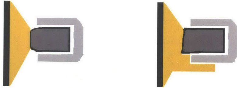
(a) Dragging due to piston movement carries oil from one region of the cylinder liner to another
