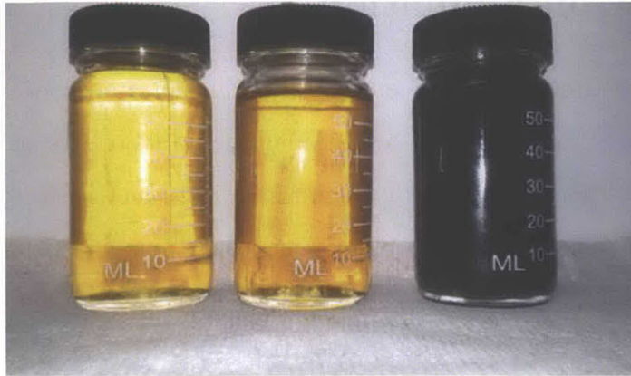
Figure 6-14: Contaminated soot oil on very right compared with clean oil on left
