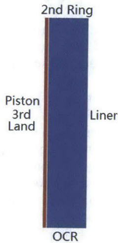
Figure 2.3 Initialization of simulation. Red color denotes oil and blue color denotes gas.
