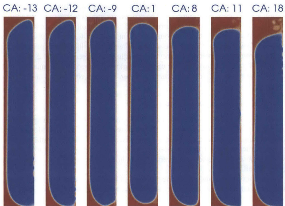
Figure 4.2 Reverse bridging in simulation, 800rpm, 0.4mm piston-liner clearance, 80 \mu m initial film
