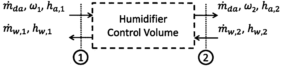
(b) Control volume in the humidifier
