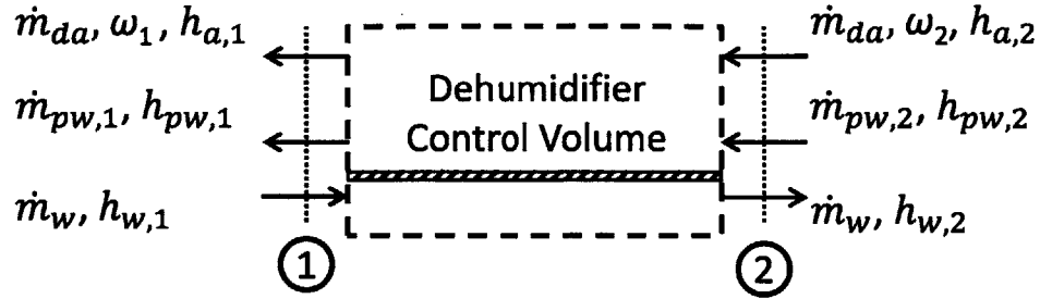
(a) Control volume in the dehumidifier
