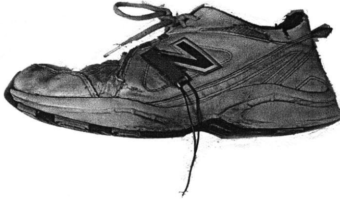
Figure 3-2: Test sneaker with macro-fiber piezoelectric energy harvesting unit attached.
