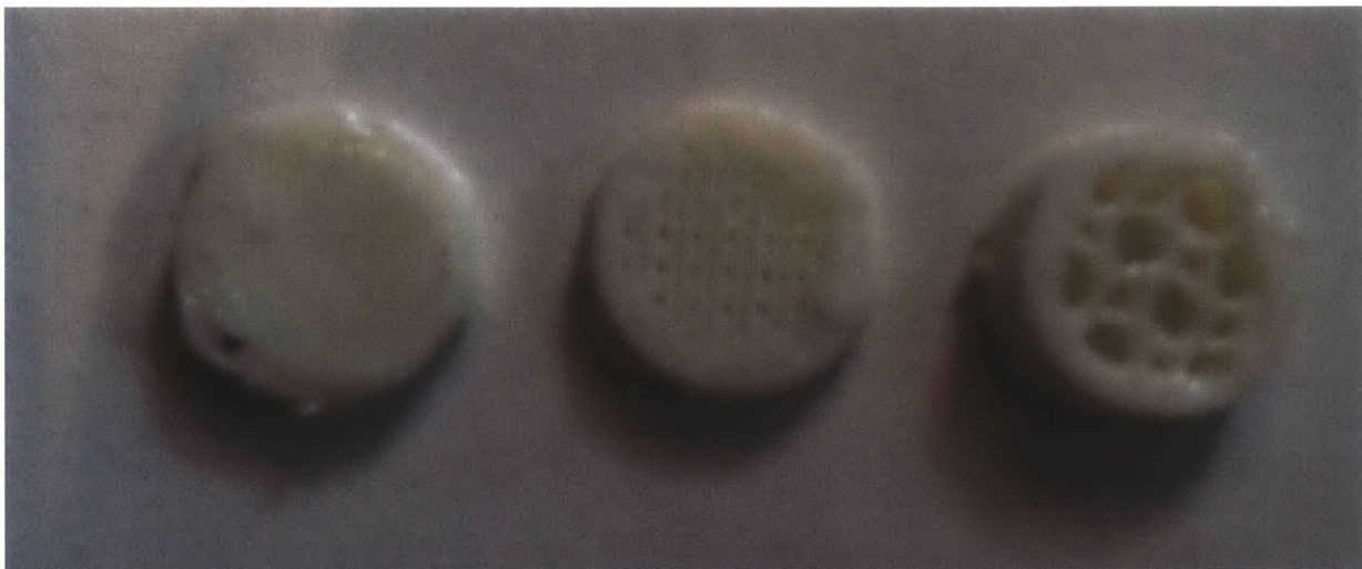
Figure 1-3. Varying Infill Scales. Above are cross-sectional views of printed components. From left to right respectively are samples printed at 100%, 50%, and 25% infill density. These samples are printed from uncolored ABS.
