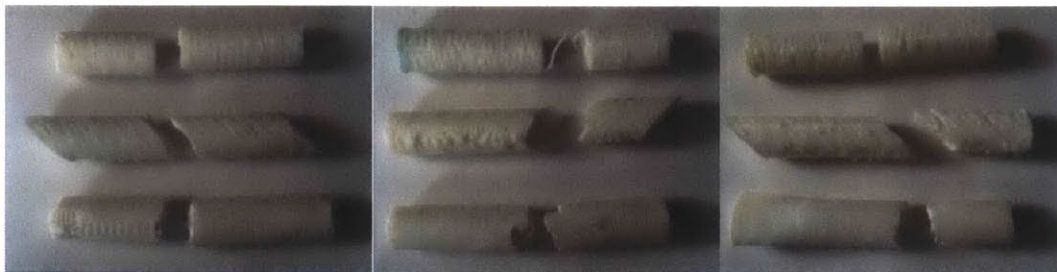
Figure 4-1. Fracture Planes of ABS Samples. ABS samples loaded in tension exhibited the above failure modes. From left to right the infill densities are 100%, 50%, 25%. Samples printed with layers perpendicular to the loading (top-most sample in each photo) failed through delamination of printed layers. Delamination almost always occurred in the elastic region of the samples. Samples printed at an angle of 45^{\circ} to the loading (center sample in each photo) failed through a combination of delamination and ductile fracture. Samples printed with loading parallel to the direction of the layers (bottom sample in each photo) failed through ductile failure.
