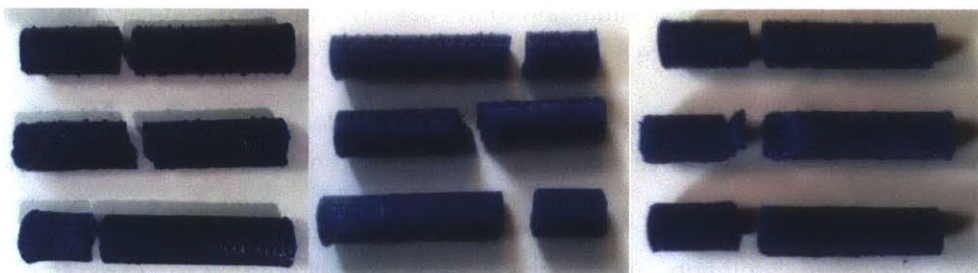
Figure 4-2. Fracture Planes of PLA Samples. PLA samples loaded in tension showed the above failure modes. From left to right the infill densities are 100%, 50%, and 25%. Samples printed with layers perpendicular to the loading (top-most sample in each photo) failed through delamination of printed layers. Delamination occurred in the elastic and plastic regions when loading these samples. Samples printed at an angle of 45^{\circ} to the loading (center sample in each photo) failed through a combination of delamination and brittle fracture. Samples printed with loading parallel to the direction of the layers (bottom sample in each photo) failed through brittle fracture.
