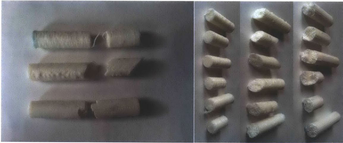
Figure B-5. Fracture Surfaces of Loaded ABS samples at 50% Infill. From top to bottom, the picture at left contains an across sample, a slant sample, and an along sample. On the right hand side are fracture surfaces of across samples, slant samples, and along samples from left to right respectively.
