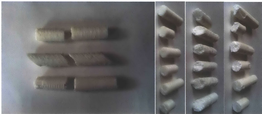
Figure B-4. Fracture Surfaces of Loaded ABS samples at 100% Infill. From top to bottom, the picture at left contains an across sample, a slant sample, and an along sample. On the right hand side are fracture surfaces of across samples, slant samples, and along samples from left to right respectively.
