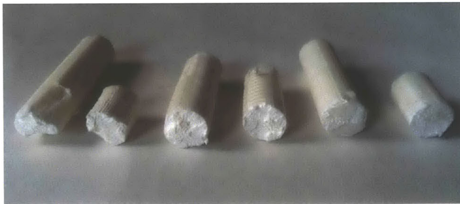
Figure 4-6. Loading Curve and Fracture Surfaces Exhibiting Ductile Fracture. Samples printed from ABS with 100% infill density and loading aligned with the layers failed through ductile fracture. These samples failed beyond the ultimate tensile strength of the part and experienced necking before failure. The line at ~35 MPa in the plot above shows the effective ultimate tensile strength. The sample is observed to reach the effective UTS and then decrease in stress as necking occurs.
