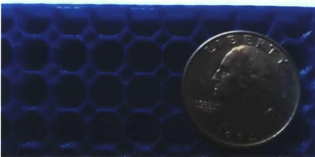
Figure 1-1. Octohedral Infill Cross Section. This image shows a cross section of a part printed with an octahedral infill pattern at 10% density. The octahedral pattern provides some strength while reducing the amount of material added.
