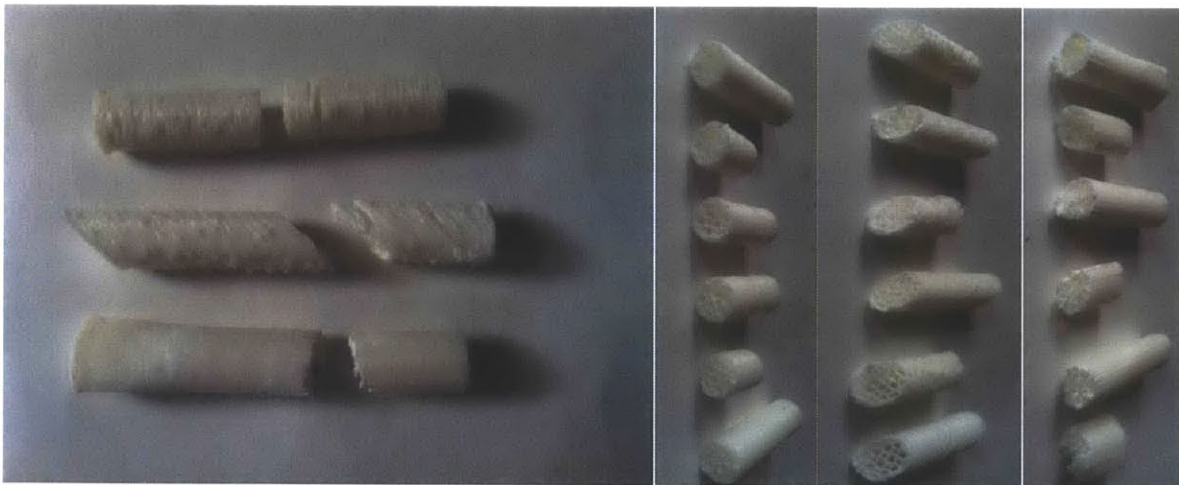
Figure B-6. Fracture Surfaces of Loaded ABS samples at 25% Infill. From top to bottom, the picture at left contains an across sample, a slant sample, and an along sample. On the right hand side are fracture surfaces of across samples, slant samples, and along samples from left to right respectively.
