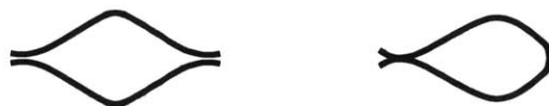
Figure 7: Cross-sectional views of the eye-shaped (left) and teardrop-shaped (right) sheet-based tube geometries.
