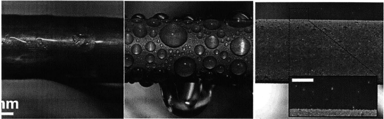
Figure 2: Filmwise condensation (L) dropwise condensation (Center) and jumping droplet condensation (R) (courtesy of Nenad Miljkovic)
