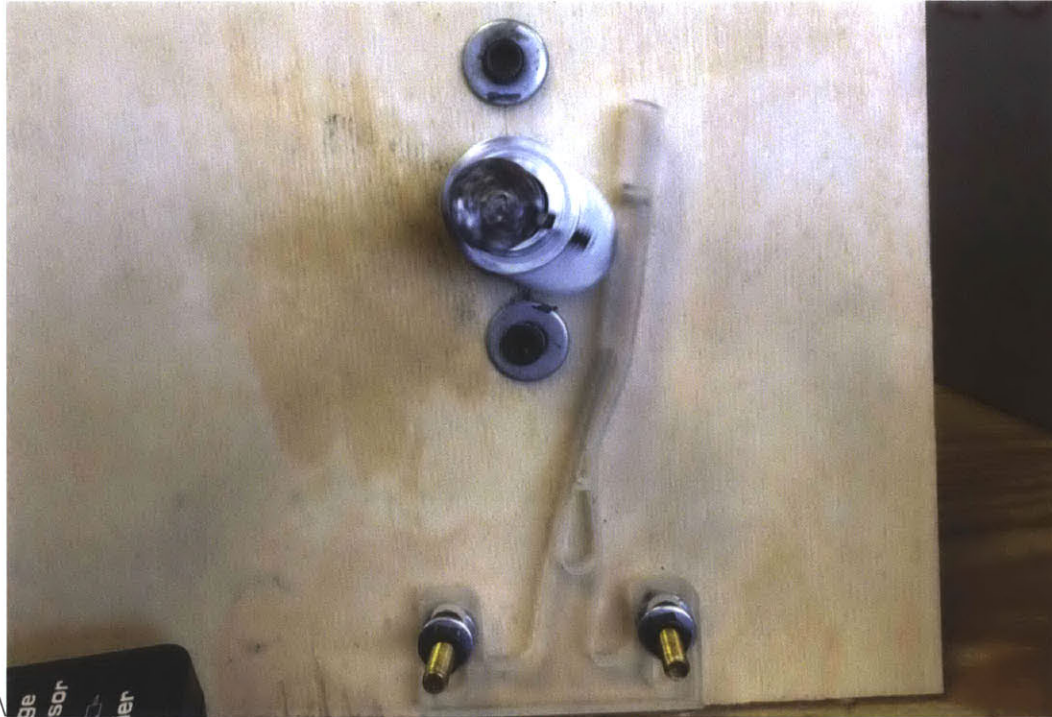
Figure 23: This is a fatigue testing using a cam that rotates between 1 and 2 Hz. Each cycle fully buckles the toothbrush truss. This simulates a user buckling the structure while brushing.
