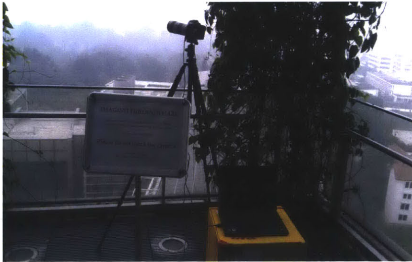
Figure 4. The experiment setup consisted of a digital SLR Canon camera setup on the 10 th floor on the CREATE building at NUS and a computer which programmed the camera to capture images.
