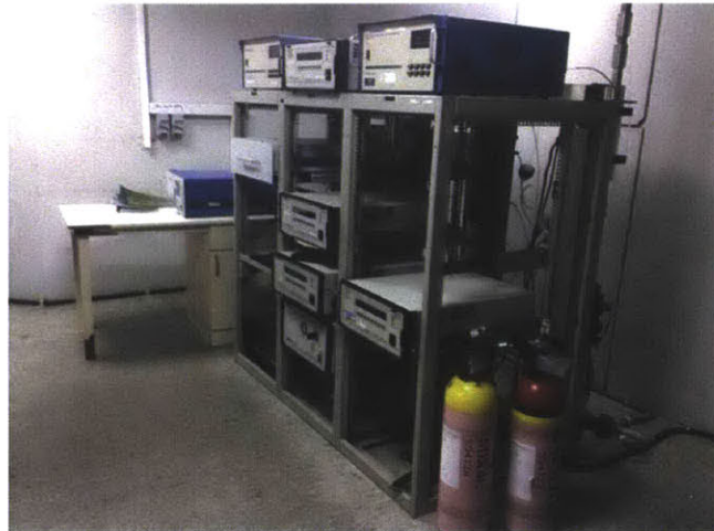
Figure 3. Haze monitor station at NEA (“How Does Singapore Measure Haze Levels?” 2014).
