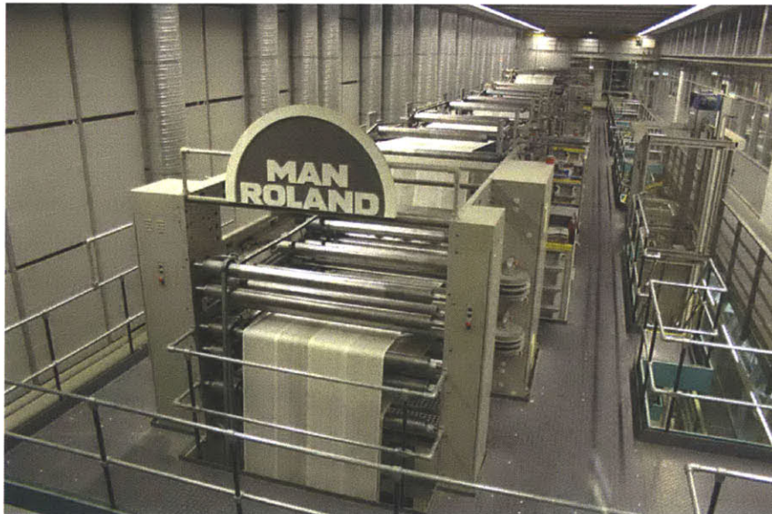
Figure 1.9: The ultimate goal is to determine how microcontact printing could be scaled up into a high-speed large-area roll-to-roll manufacturing process, such as the shown newspaper printing press.
