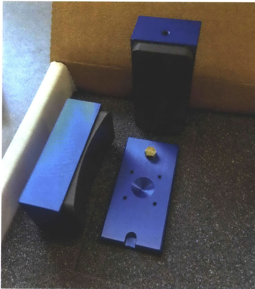
Figure 2.25: New Way radial segment air bearings with a 3" radius
