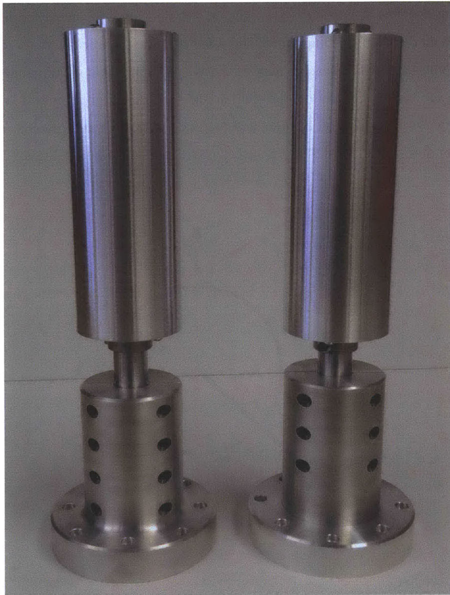
Figure 2.39: Idler rolls in flange-mounted clamps. The left mount is made from billet aluminum, while the right mount is a two-piece clamp and flange design.
