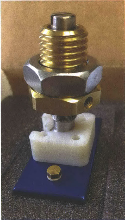
Figure 2.26: New Way radial segment air bearing (blue) mounted on a fine pitch ball-head screw in a brass mounting nut (gold). The 3D printed retaining block (white) is used to keep the air bearing connected to the screw.
