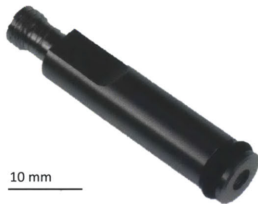
Figure 4-6: The pipe that allowed fluid communication between the two nozzle blocks, with the O-ring installed.
