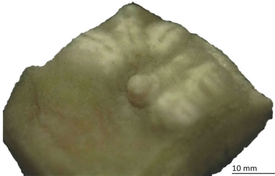
Figure 5-11: Cuts made on a sample with fat and muscle produced whitening. These cuts were shallower and narrower than cuts made in dermis-only samples: one measured an average depth of 0.4 mm with a standard deviation of 0.2 mm, and an average width of 1.8 mm with a standard deviation of 0.4 mm.
