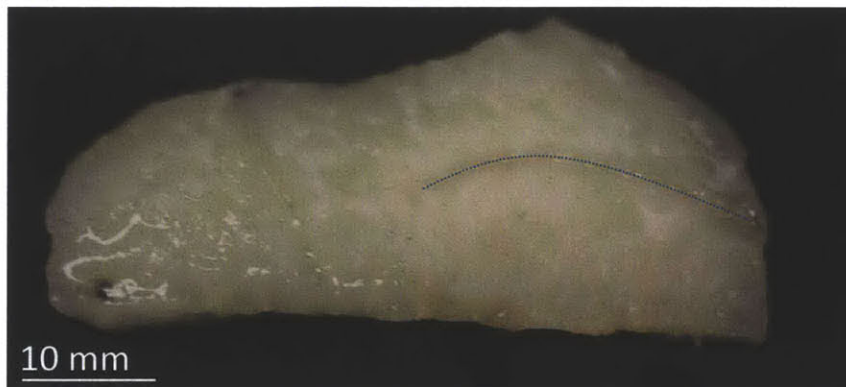
Figure 5-14: Cut made with blade pre-cut. Blue dotted line traces the cut path.
