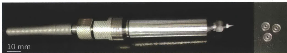
Figure 3-7: The single nozzle debrider wand. On the right are the acrylic crush washers that created a watertight seal between the ceramic nozzle and the debrider base.
