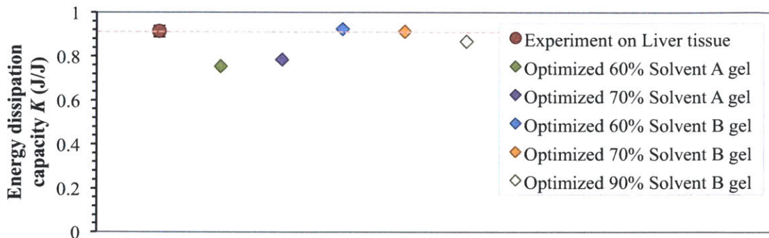
Figure 4.22: Comparison of energy dissipation capacity K for the optimized gels with Solvent A and Solvent B against rat liver tissue (Impact velocity v_{in} = 8.2 mm/s)
