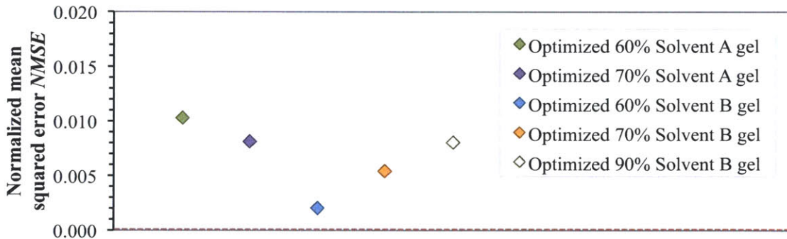
Figure 4.21: Comparison of normalized mean squared error NMSE for the optimized gels with Solvent A and Solvent B against rat liver tissue (Impact velocity v_{in} = 8.2 mm/s)
