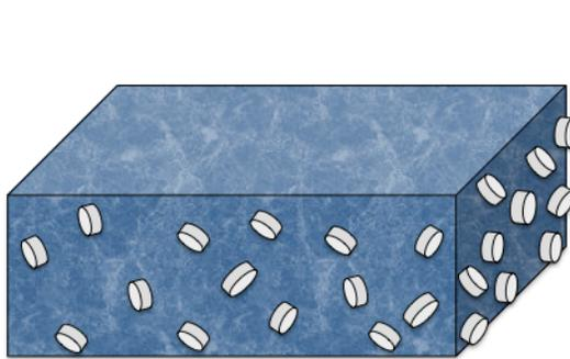
**Step 3:** Heat press to remove pores
