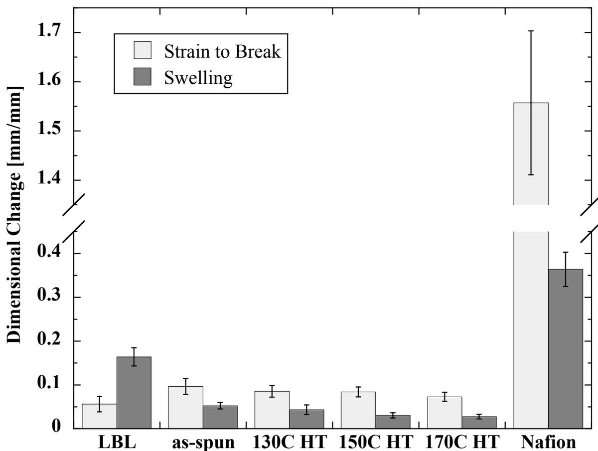
**Figure 5.** Dimensional change in the strain to break (at 50% RH) and linear swelling of composite PEMs and Nafion.
