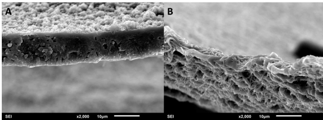
Figure 4. Representative SEM micrographs of composite LbL-electrospun fiber membrane fracture surfaces: A) “dry” membrane fracture plane indicating brittle fracture mechanism, B) “wet” membrane fracture plane showing thinning & plastic deformation during ductile rupture. The scale bar for each image is 10  $\mu\text{m}$ .
