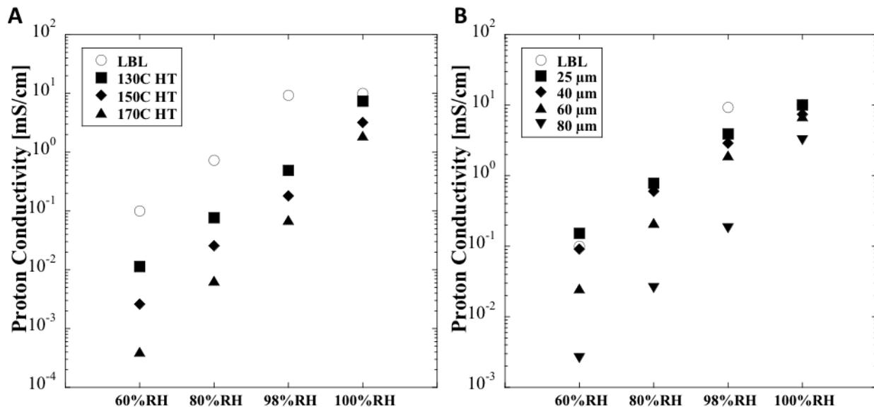
**Figure 7.** Humidity dependence of the proton conductivity of (A) the composite PEMs assembled on various thermally treated EFMs (80  $\mu\text{m}$  thick before annealing) and free-standing LbL film and (B) the proton conductivity for different composite PEM thickness [150  $^{\circ}\text{C}$  heat-treated samples].
