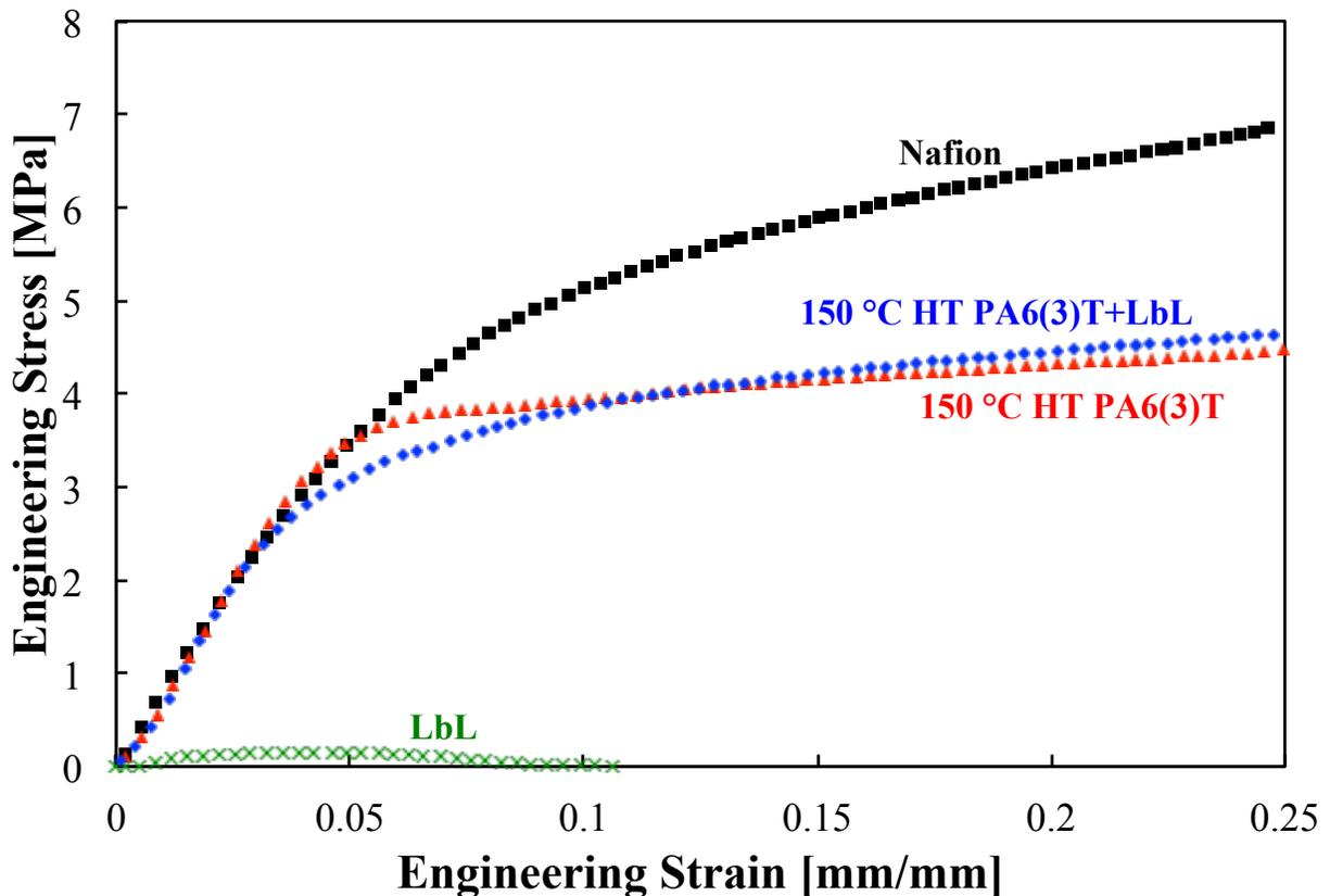
**Figure 3.** Representative stress-strain plots for hydrated membranes of: Nafion (black squares), 150 °C heat-treated PA 6(3)T nanofiber mat (red triangles), free-standing LbL film (green x's), and the composites of PA 6(3)T and using 150 °C heat-treated electrospun mat (blue diamonds).
