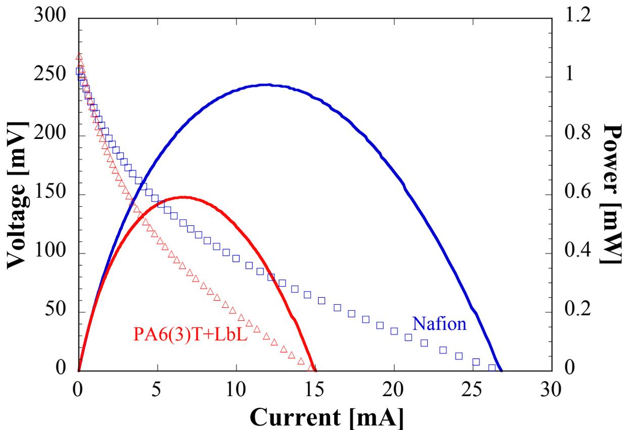
**Figure 8.** V-I polarization curves for Nafion and PA6(3)T+LbL composite membrane using Pt catalyst for both the anode and cathode GDL in 10 wt.% methanol/water mixture.
