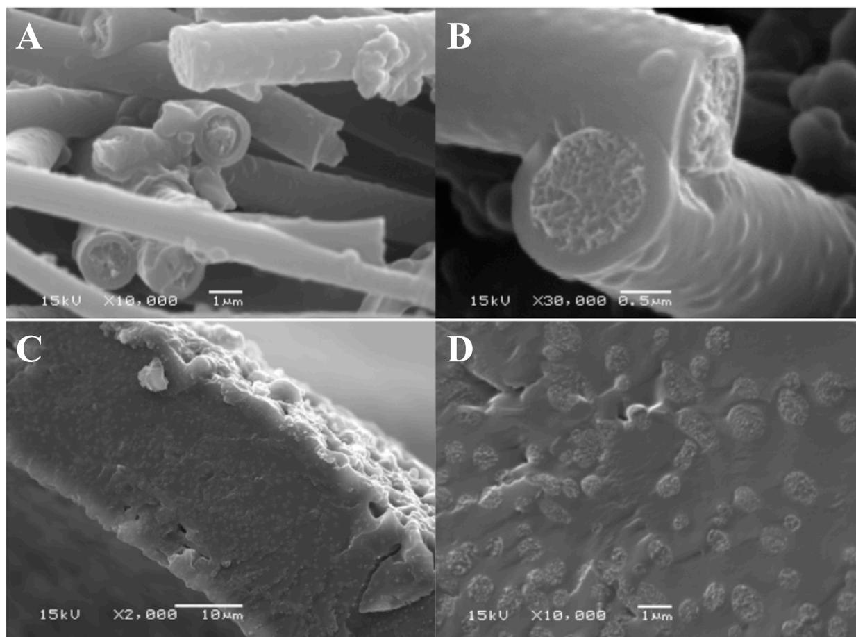
**Figure 2.** SEM micrograph of ~800 nm diameter PA 6(3)T fibers coated with 50 bilayers of PDAC/sPPO (A & B). SEM Micrograph of composite PEM, consisting of PA 6(3)T fibers whose interstices are completely filled with PDAC/sPPO (250 BLs with vacuum assist) after being hot-pressed while hydrated. Scale bars for A & D are 1 μm; scale bar for B is 0.5 μm; scale bare for C is 10μm.
