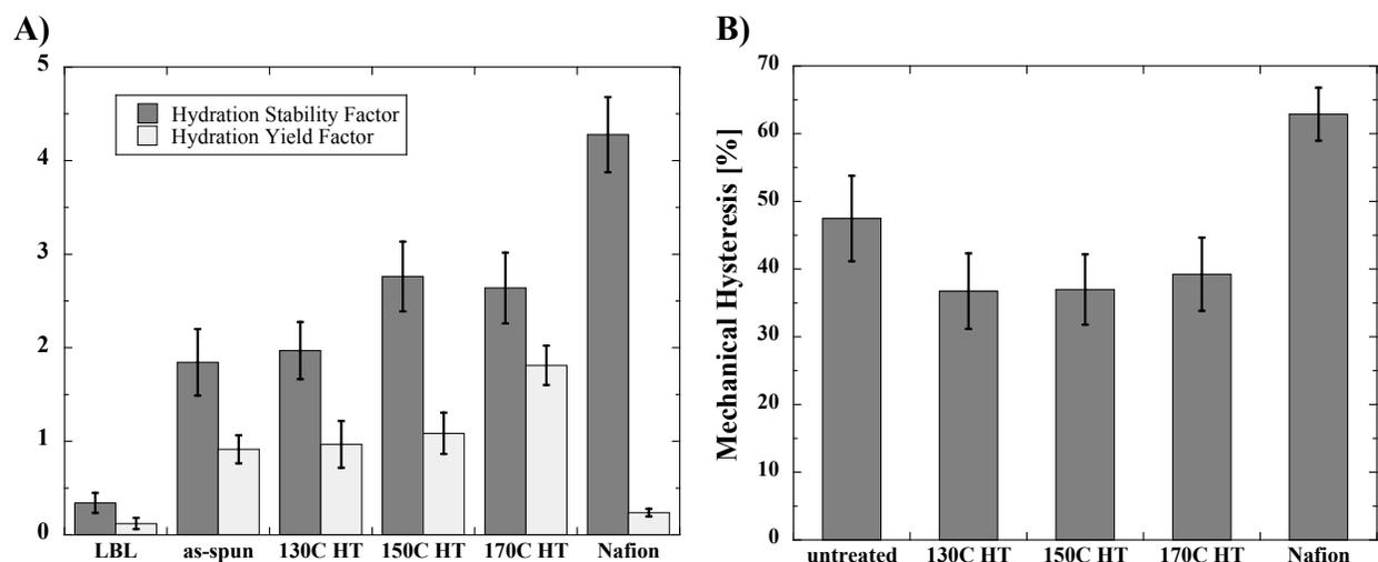
**Figure 6.** (A) Comparison of hydration stability factor and hydration yield factor for the free-standing LbL film, composite PEMs made with EF mats annealed at different temperatures, and Nafion. (B) Comparison of the mechanical hysteresis for composite PEMs made with EF mats annealed at different temperatures and Nafion.
