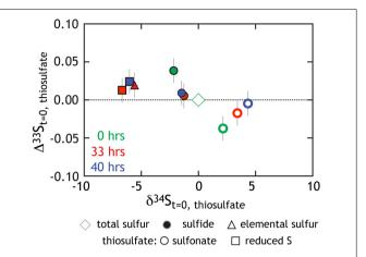
FIGURE 5 | Triple isotope data for thiosulfate reduction experiments. As opposed to Figure 4B where we presented calculated  $^{34}\epsilon$  values, here all isotope data is normalized to the bulk composition of the starting thiosulfate (green diamond at origin). Also in green are the site-specific compositions of the reduced and sulfonate S (square and circle, respectively). Those same S sites at times 33 h (red) and 40 h (blue) are also included.
