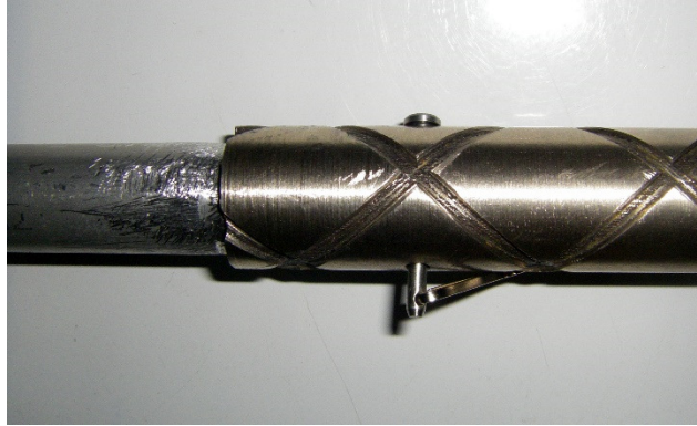
FIGURE 5-3: UPDATED CONNECTION BETWEEN THREADED ROD AND ALUMINUM ROD
