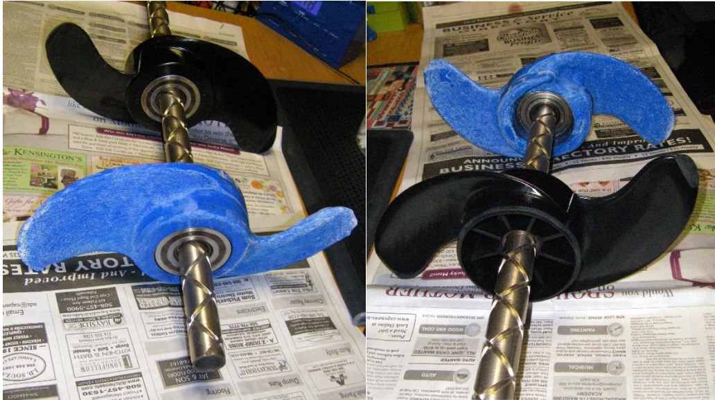
FIGURE 4-16: ASSEMBLY PROPELLER ASSEMBLY (PROPELLER, ONE-WAY CLUTCH BEARING, THREADED NUT) USING LOCTITE
