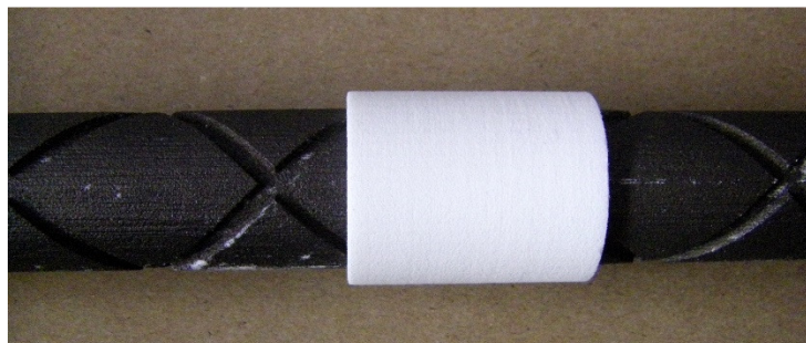
FIGURE 4-6: STAINLESS STEEL PRINTED ROD WITH PLASTIC NUT
