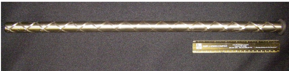
FIGURE 4-8: TURNED DOWN 3D PRINTED STAINLESS STEEL THREADED ROD
