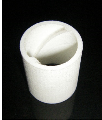
FIGURE 4-4: PLASTIC 3D PRINTED THREADED NUT
