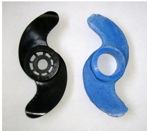
FIGURE 4-12: ORIGINAL AND PRINTED PROPELLER AFTER MACHINING
