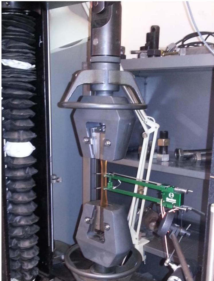
Figure 3.5: Specimen setup in the Instron with extensometer.
