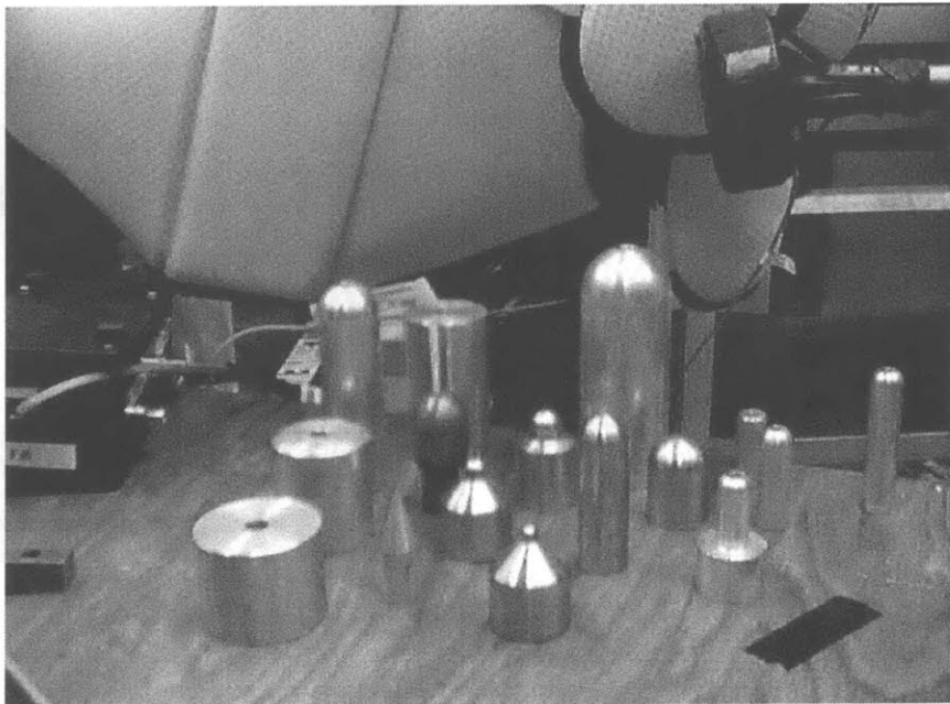
Figure 7. Interchangeable tups for impactor unit of FRED.
