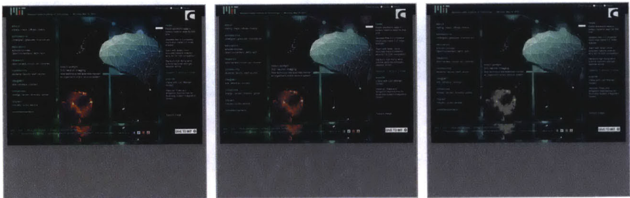
Figure 11. [left] The raw image conversion from mit.edu [middle] The quantized image of mit.edu represented by 10 colors [right] The quantized image of mit.edu represented by 5 colors
