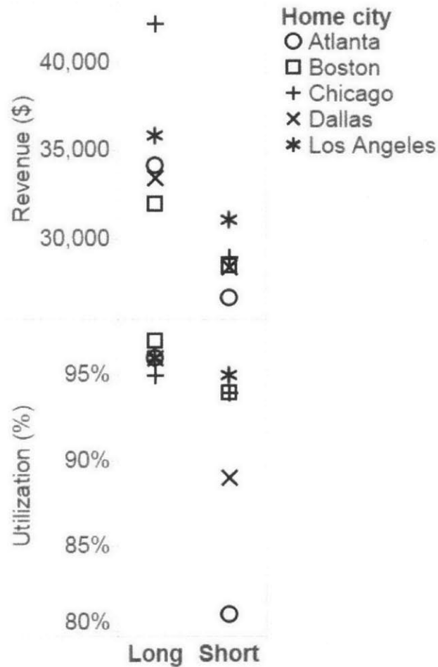
Figure 13 Comparison of revenue ($) and utilization (% loaded) for long-haul preference and short-haul preference for the August simulation run. In the long-haul condition, the longest haul in the dataset is given the highest ranking; the opposite is true for the short-haul strategy.
