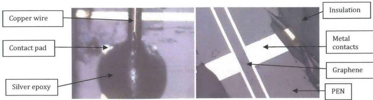
Figure 11: a) Optical image of the manual wirebonding. b) Schematic illustration of a graphene-on-PEN solution-gated transistor.
