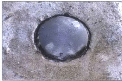
SFpark embedded parking space sensor and smart parking meters
