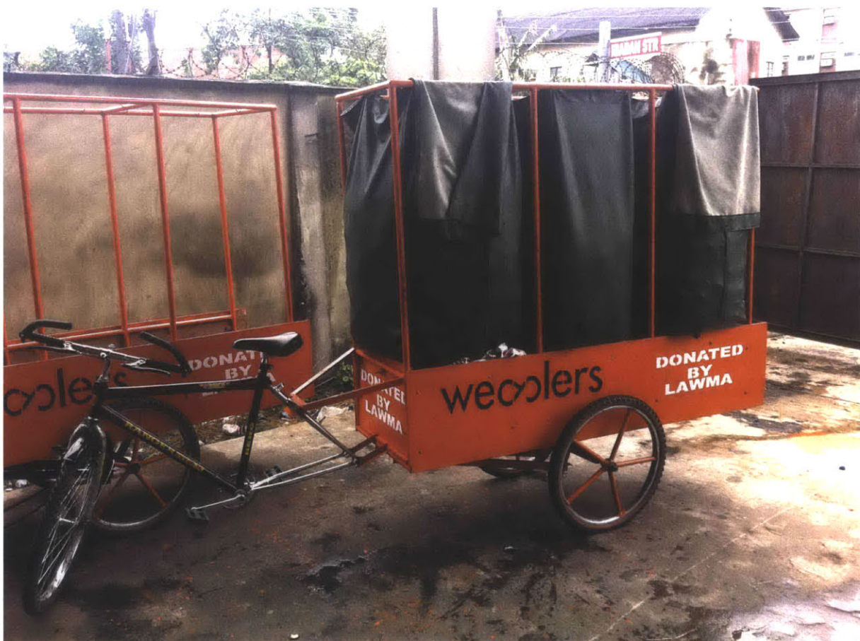
Figure 1-1: An existing WeCycle. The rear chassis is sectioned with canvas bags to hold three different types of materials. Photo credit: Billikiss Adebiyi-Abiola.
